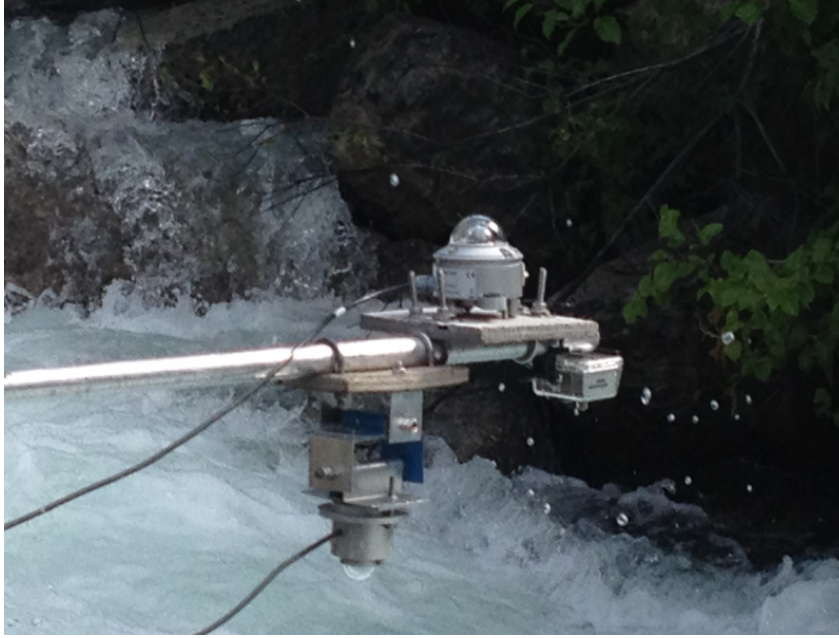
Figure 2.3: Monitoring set-up used to measure albedo and obtain camera imagery mounted at the end of the horizontal support pole.
