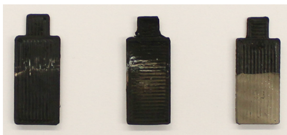
Figure 3.2 Electroplating comparison on 3D-printed electrodes. Left: Reprapper Conductive ABS, Middle: MatterHackers Conductive ABS, Right: Proto-Pasta conductive PLA.
