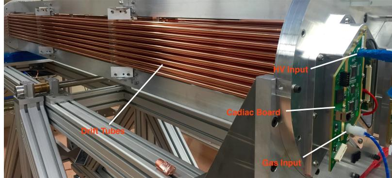
Figure A.1: Straw prototype with Gas and HV Input Connected
