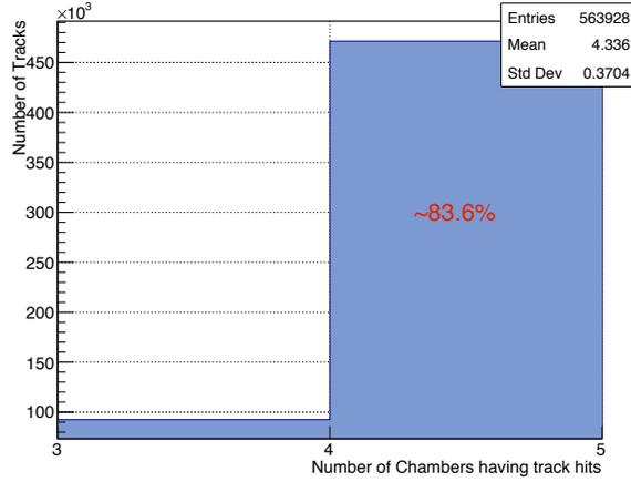
Figure 4.1: Number of straw chambers hit by downstream track.
