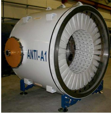
Figure 2.13: Here is the first LAV station which has 5 rings of OPAL lead glass blocks. The glasses are wrapped.
