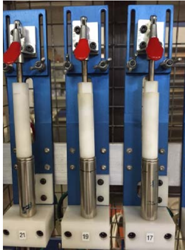
Figure 3-1. Cell holder for cell testing. The three metallic cylinders in the bottom half of the photo are the 30U cylindrical lithium ion cells.
