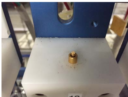
Figure 3-3. Bottom portion of the cell holder, showing the spring-loaded center pin for current conduction, and outer metallic tube for voltage measurement.
