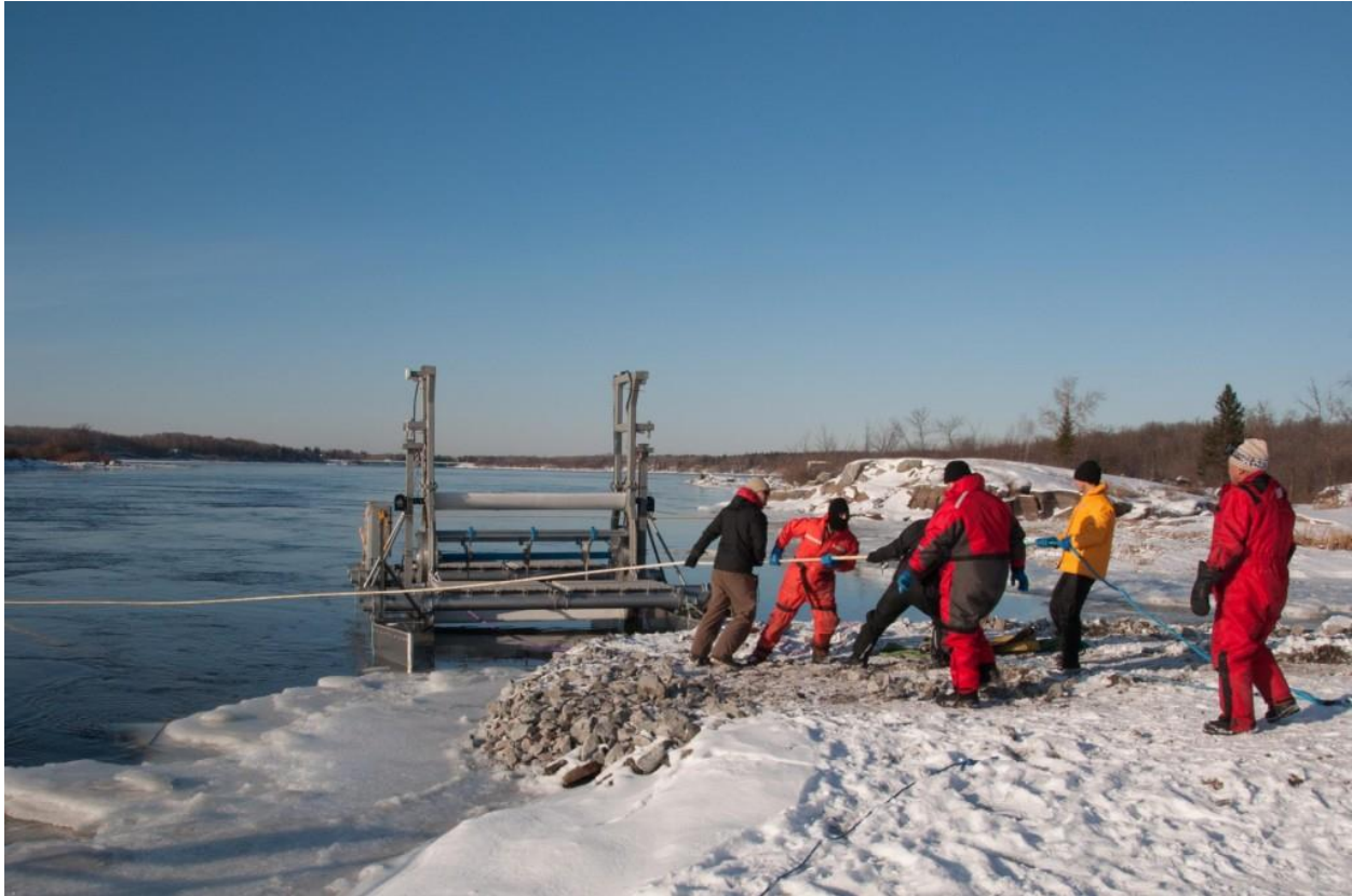
Figure 2-11: Mavi Innovations Mi1 22KW floating style turbine. Reprinted with permission from Mavi Innovations Inc., source: http://mavi-innovations.ca/technology/
