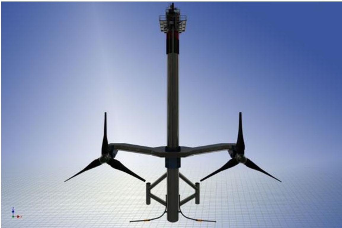
Figure 2-7: Seagen "S", 1.2 MW turbine in generation mode. The turbines are positioned below the water but can be raised above it for maintenance. The piling structure is "pinned" into the seafloor. The structure also has an active sonar type marine animal avoidance device which will stop the turbine blades if a signal return is detected with a certain proximity to the device. Reprinted with permission of Atlantic Resources Limited, source: www.marineturbines.com .
