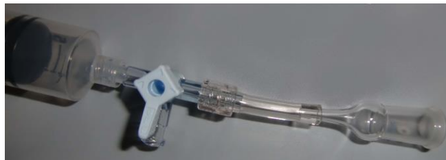
Figure 8. Suction device: syringe 30 mL, three-way stopcock, silicone tubing and glass suction cup.
