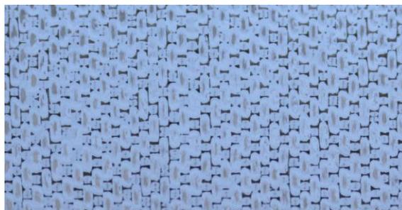
Figure 2.4: Surface porosity (black) on a small, flat prepreg laminate.
