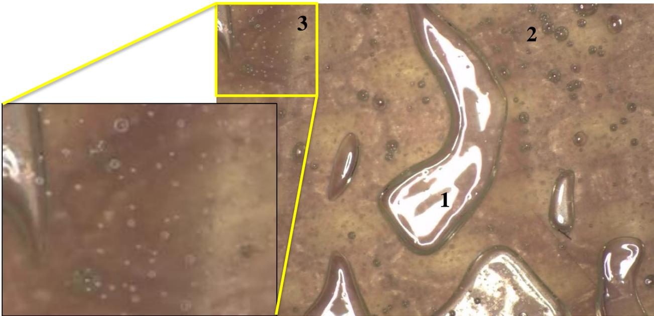
Figure 3.6: In-situ image of 75% RH neat resin at 0.49 atm; 50X magnification, image size 6901 x 4927  $\mu\text{m}^2$ .
