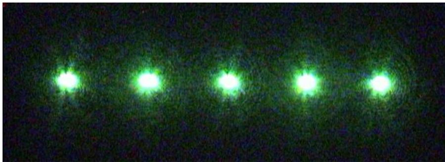
Figure 5.8: Five particles simultaneously trapped in a CPBB optical trap, demonstrating optical binding.
