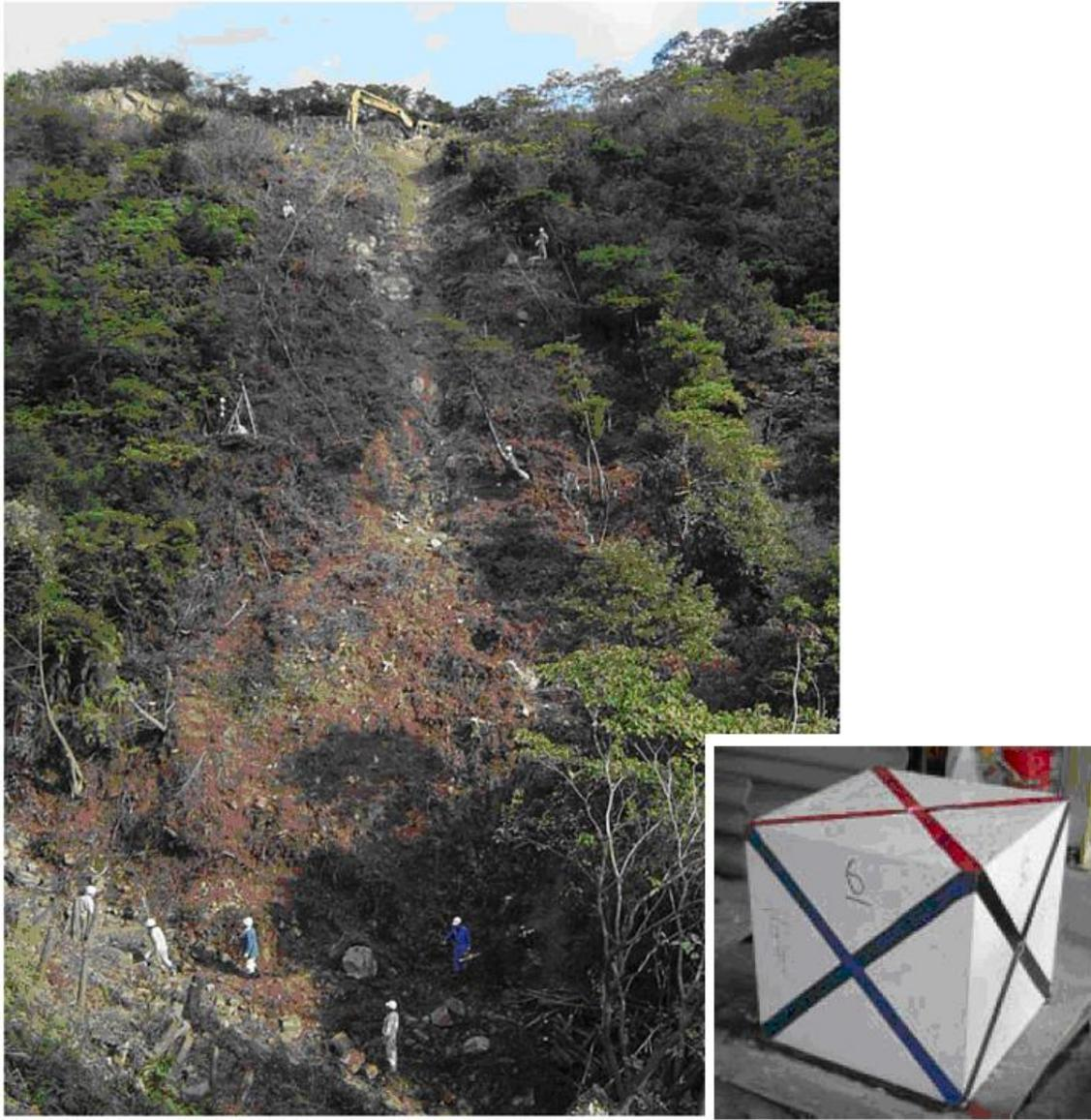
**Figure 2.5: Ehime test site in Japan – rock slope with talus deposit at base; concrete cube test block**
