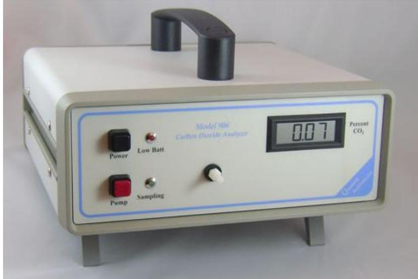
Figure 3-1 Model 906 CO<sub>2</sub> analyzer
