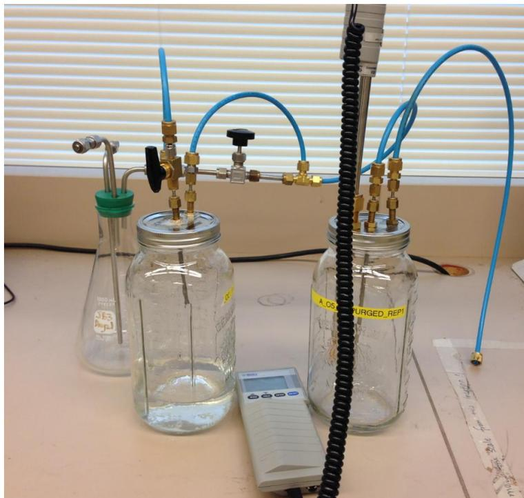
Figure 4-21 Humidifier setup
