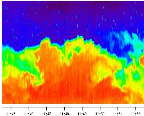
**Figure 1.1:** Lidar backscatter image of the CBL (property of Shane D. Mayor, Department of Geological and Environmental Sciences, California State University). Time is on the bottom axis, backscatter intensity is represented by the colours red-blue. Red corresponds to high intensity, and therefore high aerosol concentration. Regions with negligibly low concentrations are dark blue.
