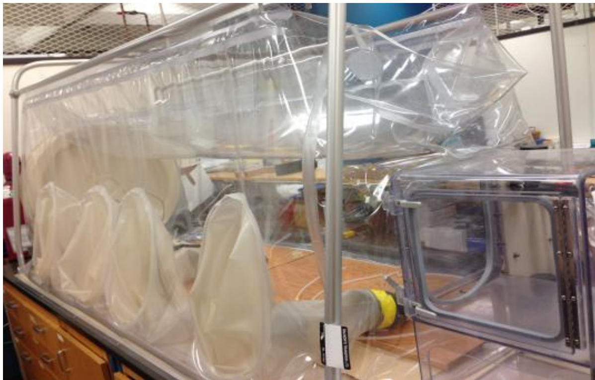
Photo1: Vinyl glove box. SEPs were performed in vinyl glove box under anaerobic condition. To create anaerobic condition, the glove box was purged with a mixture of pure N_2 and N_2/H_2 until O_2 was below 2% in the chamber.
