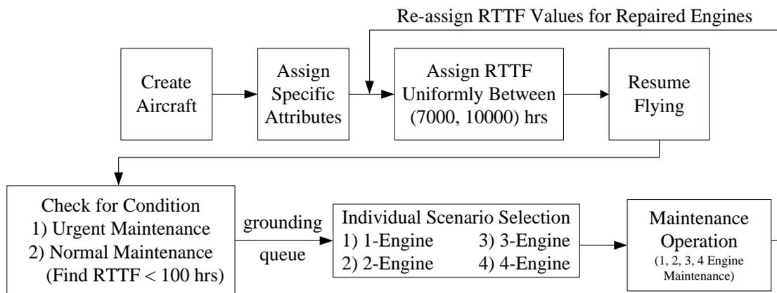
Figure 4.1: Maintenance Operation for “Fixed” Number of Engines
