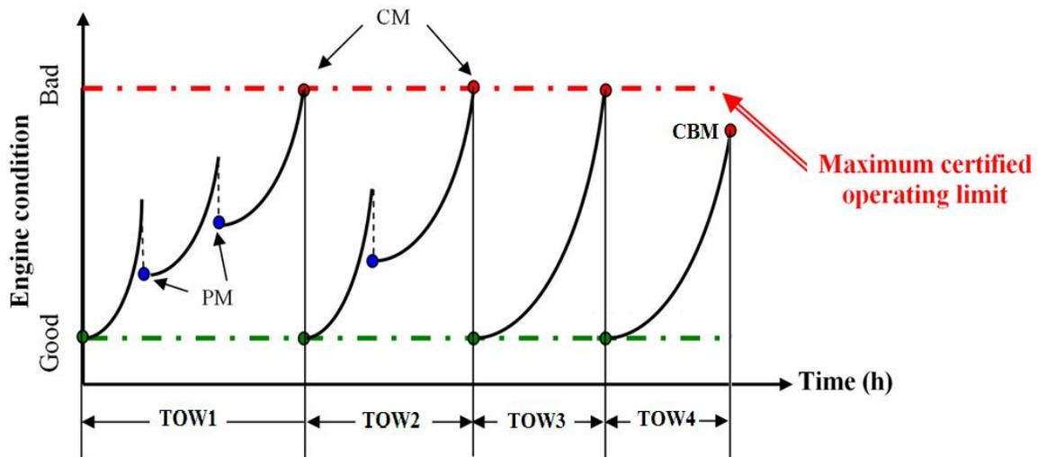
Figure 2.2: Engine Condition and Time-on-Wing Characteristics
