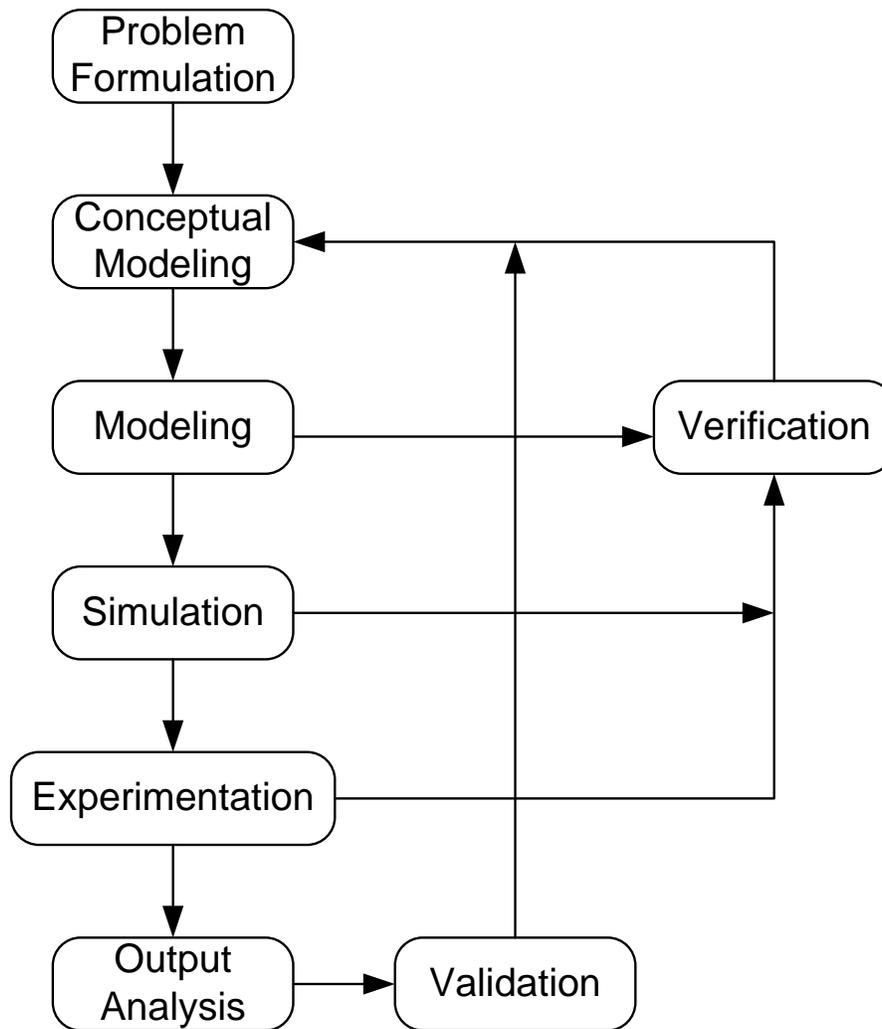
Figure 3.1: Schematic Block Diagram of Simulation Process
