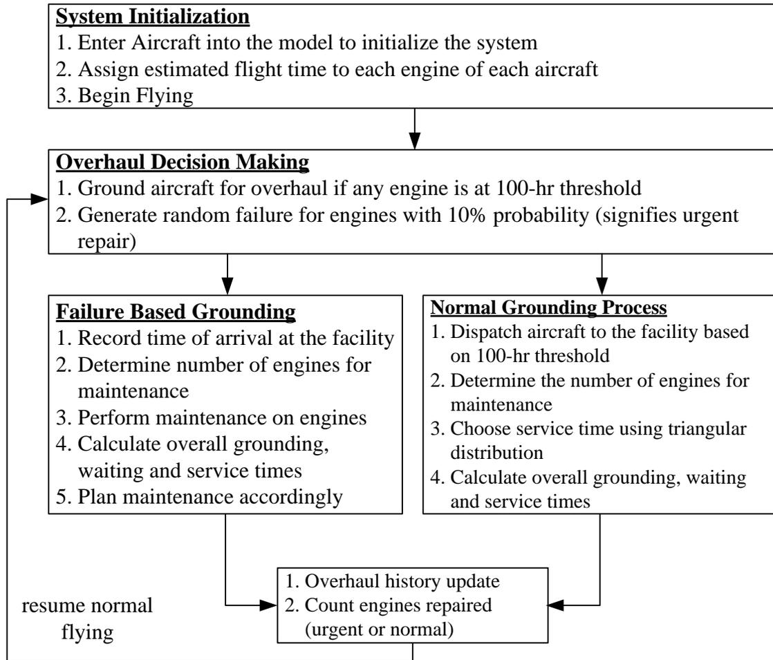
Figure 3.4: Simulation Model for Engine Maintenance
