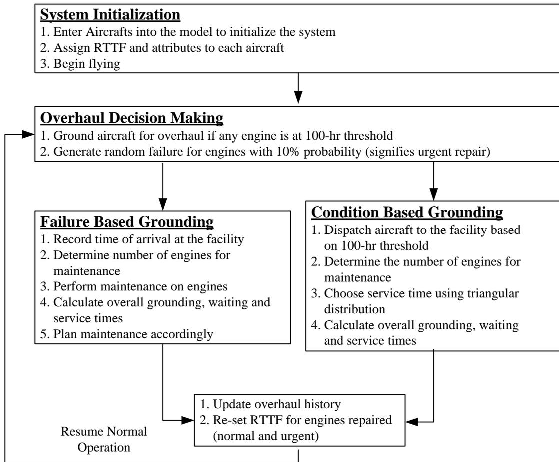
Figure 4.11: Overall Maintenance Procedure Flow Diagram
