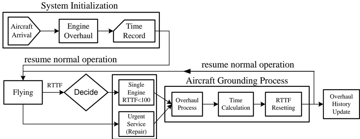
Figure 3.5: Block Diagram for 1-Engine Maintenance
