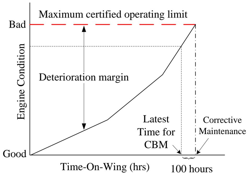
Figure 1.3: TOW Graph Representing Engine Deterioration
