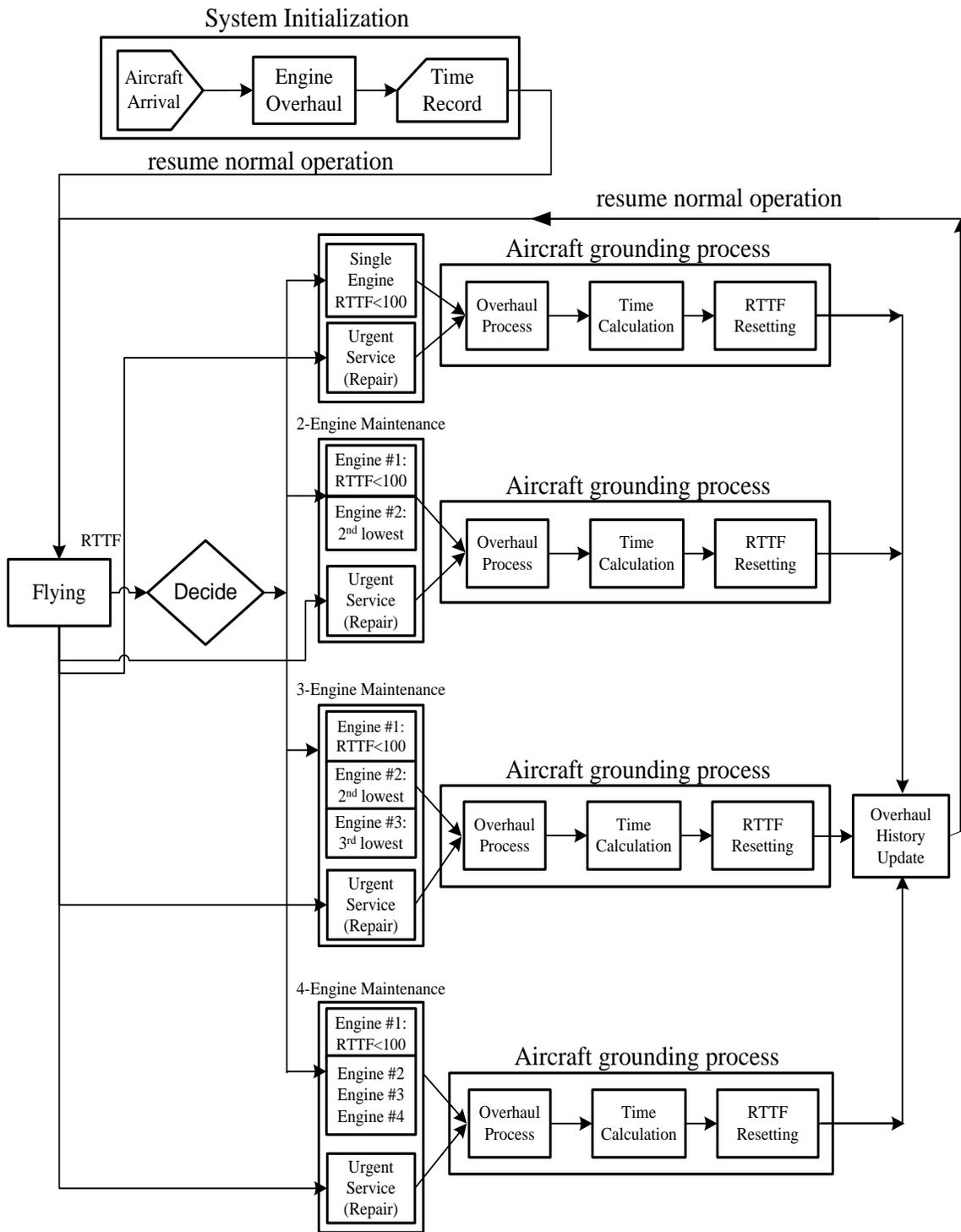
Figure 3.9: Block Diagram for ISS Engine Maintenance
