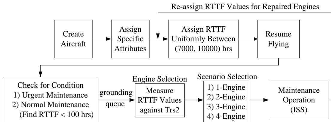
Figure 4.2: Graphical Representation of Maintenance Operation for ISS
