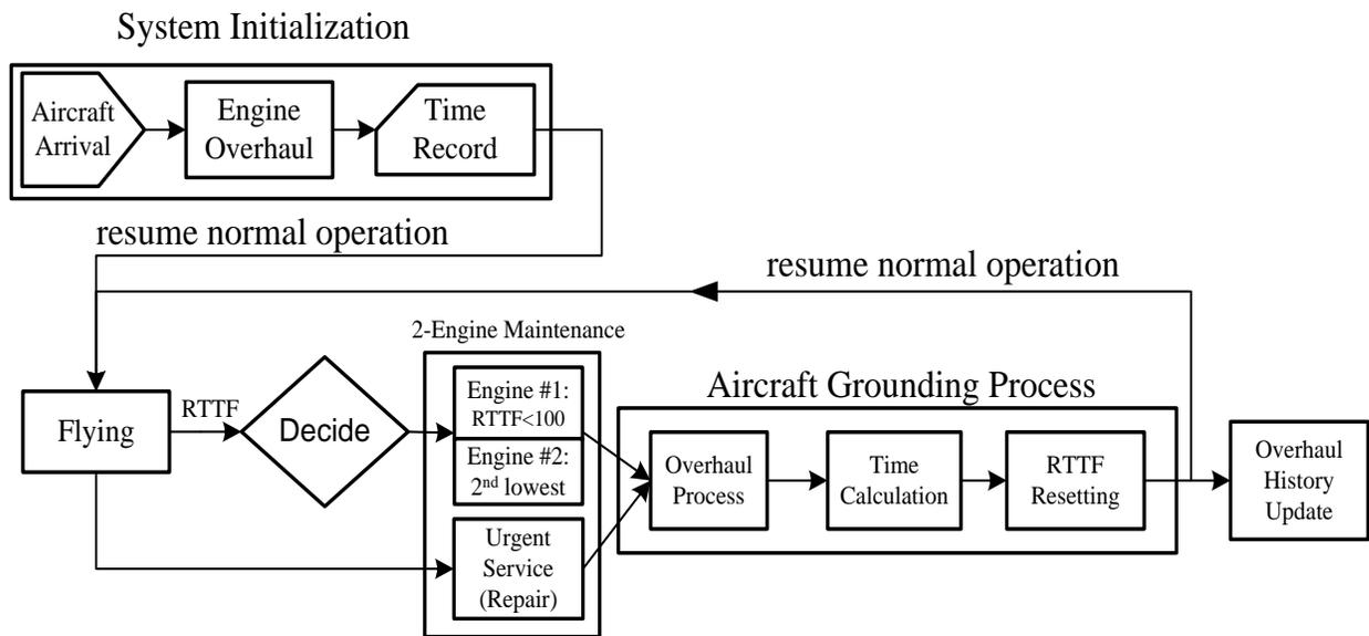
Figure 3.6: Block Diagram for 2-Engine Maintenance
