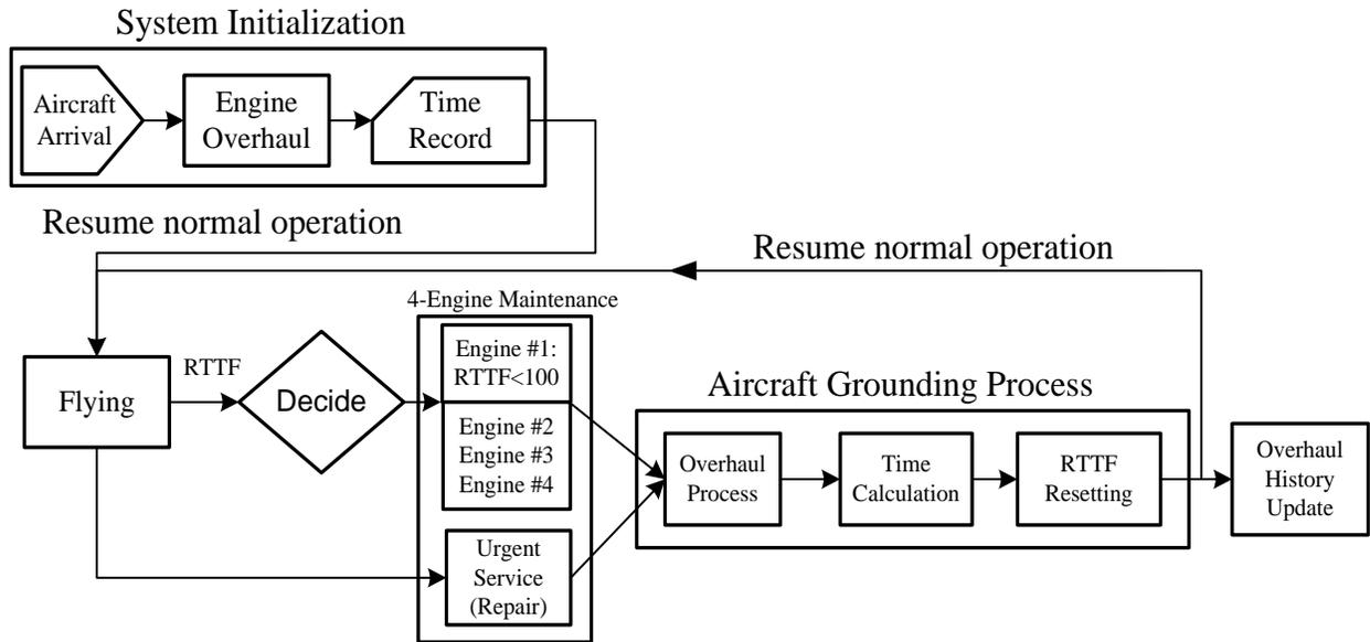
Figure 3.8: Block Diagram for 4-Engine Maintenance
