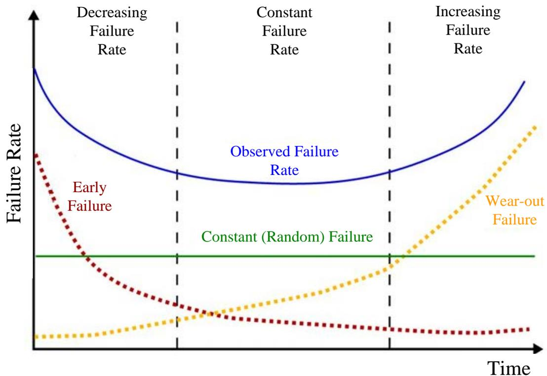
Figure 1.1: Component Failure Rate over Time
