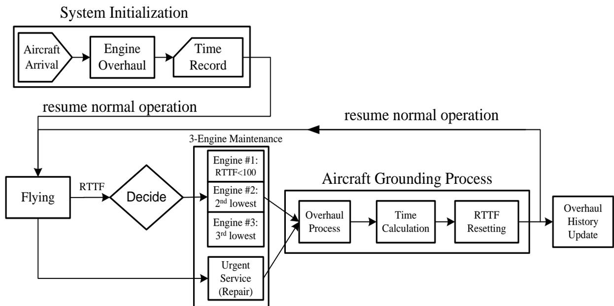
Figure 3.7: Block Diagram for 3-Engine Maintenance
