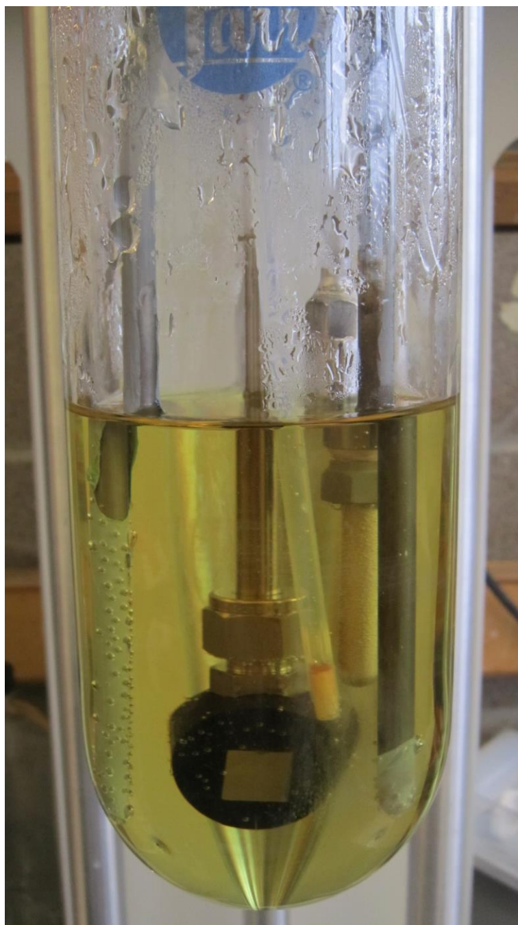
Figure A-2 Inside of the glass reactor for high temperature high pressure autoclave.
