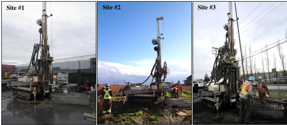
Figure 3.15 Conventional rotary mud drilling at Site #1, # 2, and #3 for obtaining relatively undisturbed soil samples
