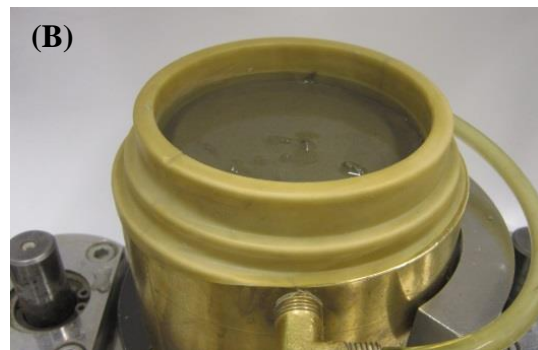
(B) Reconstituted specimen placed in the wire reinforced membrane
