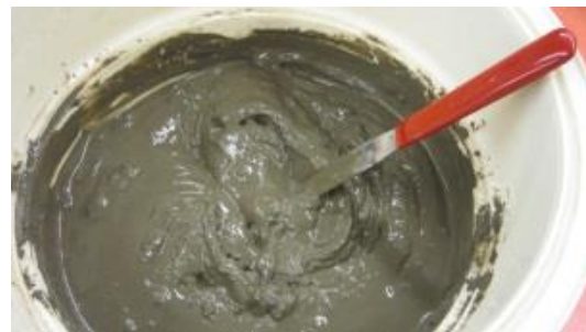
(B) Mixing of soil with de-aired water
