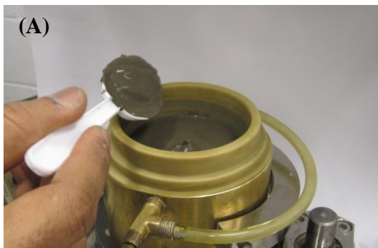
(A) Spooning the slurry to the cavity surrounded by the wire reinforced membrane
