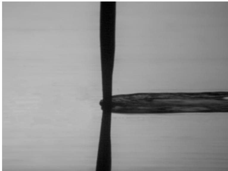
Figure 3-33 Non-Newtonian behaviour of Simu liquid jet
