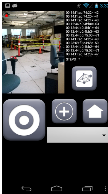
Figure 2.6: A screen shot of the data collection application used to generate training and evaluation datasets for localization.
