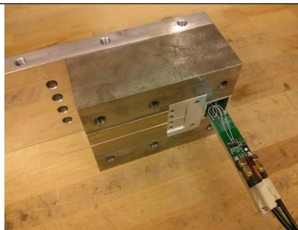
**Figure 5-28 - PCB assembly inserted into aluminum receptacle**
