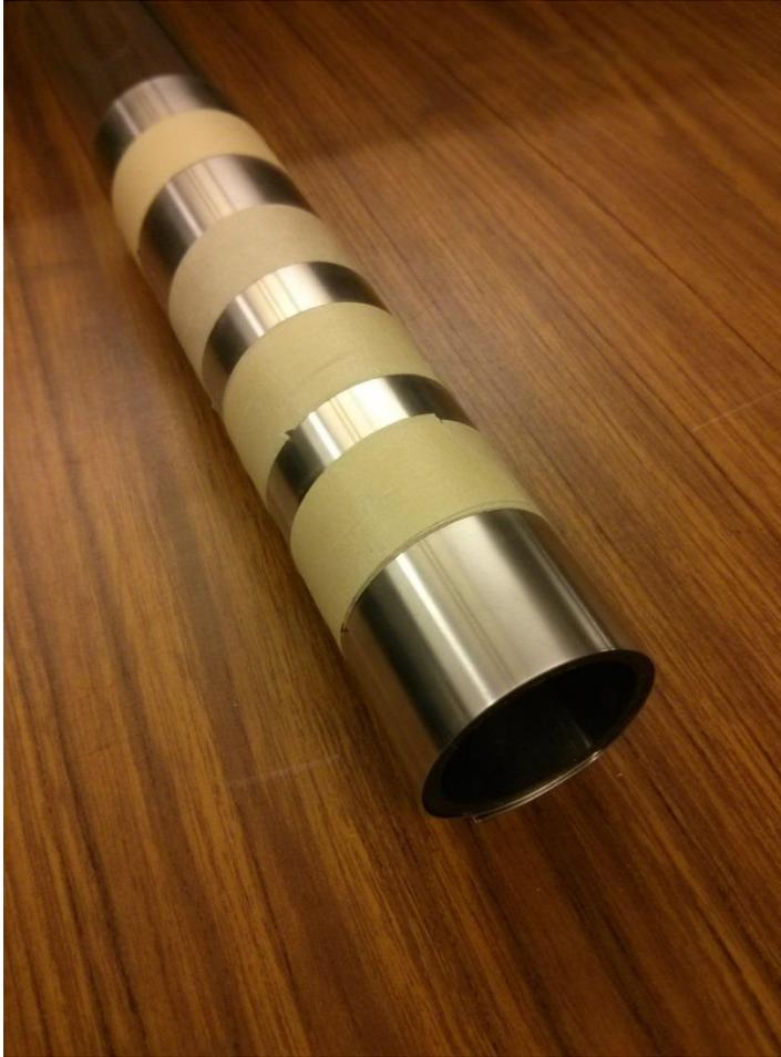
**Figure 5-3 – Zero magnetic reference field consisting of mu-metal wrapped around a plastic tube**
