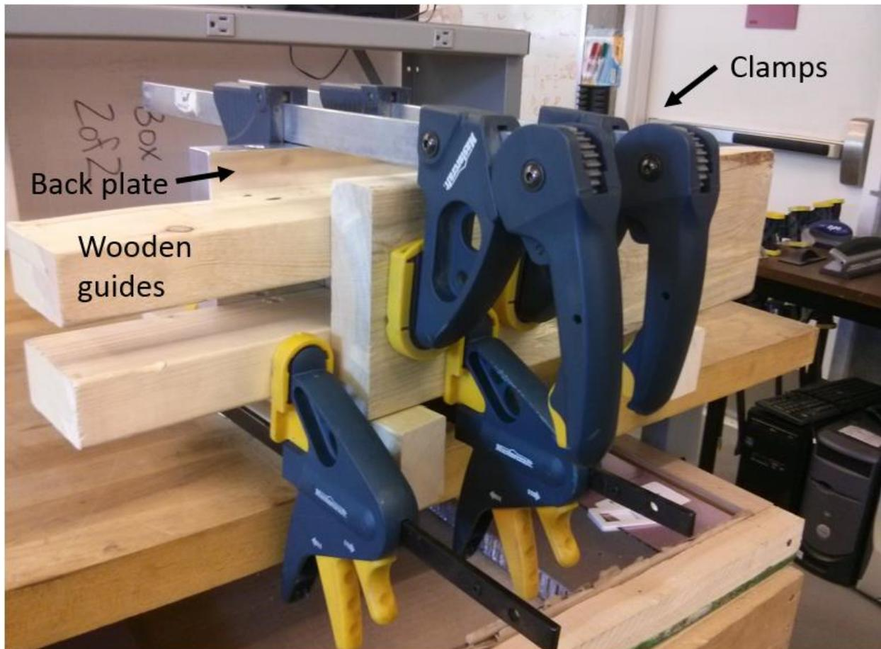
**Figure 5-19 - Temporary wooden guides for inserting the magnets into the magnetic field source**
