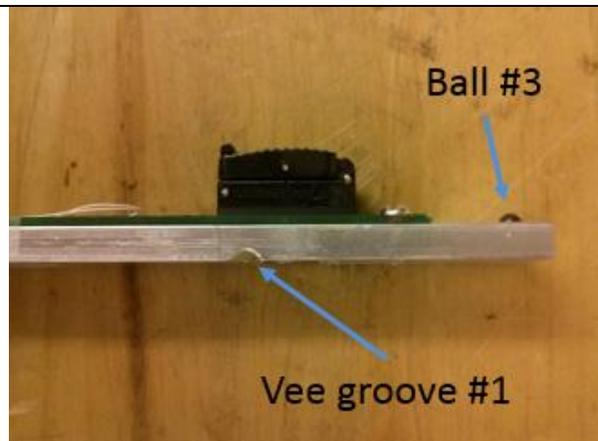
**Figure 5-26 - Side view of PCB base showing ball and grooves for kinematic coupling**
