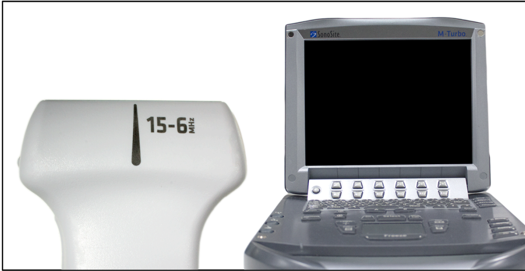
Figure 8: Portable Ultrasound machine and the linear transducer used for imaging the models.
