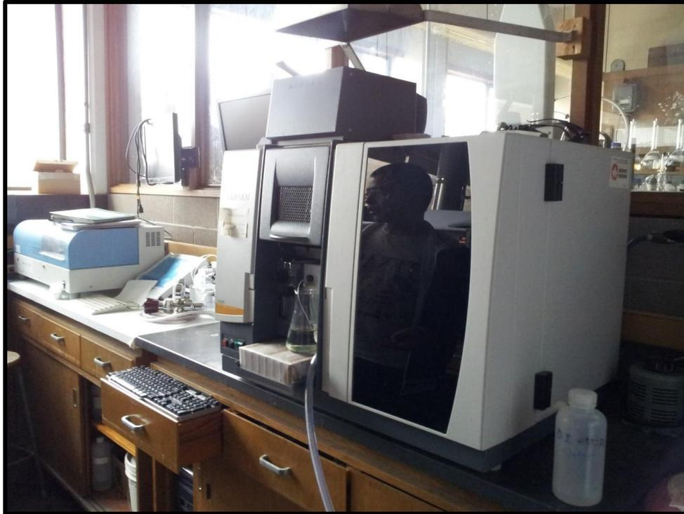
**Figure 4.5 Atomic Absorption Spectroscopy used to analyze liquid samples**
