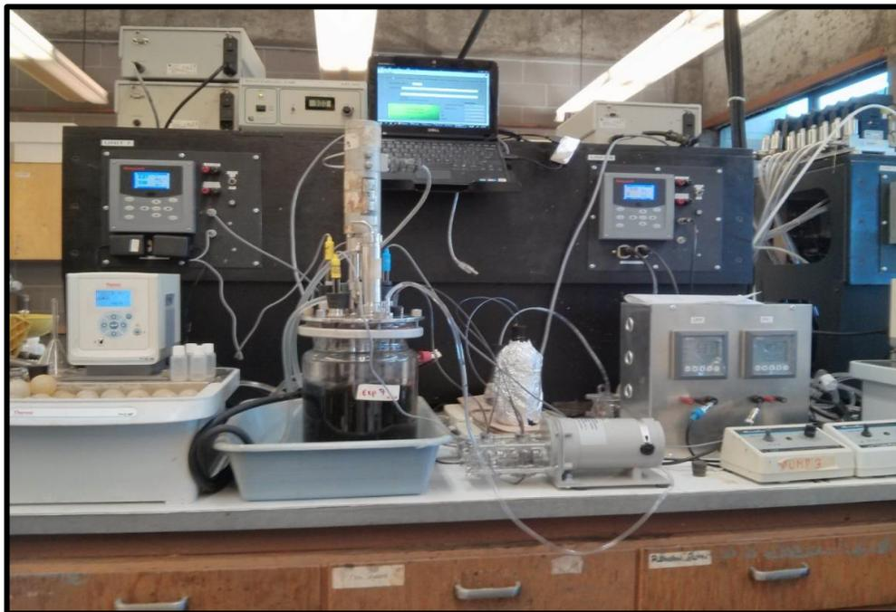
**Figure 4.4 Typical Equipment Set-up for Permanganate as oxidant**
