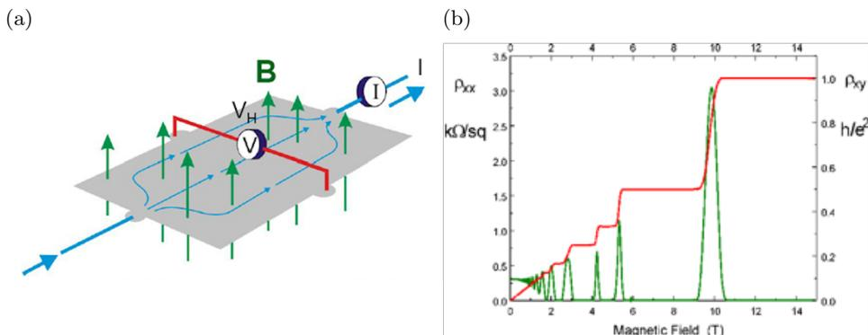
Figure 1.1: (a) Experimental setup for the Quantum Hall effect. (b) Plateaus observed at integer values of the Hall resistivity
