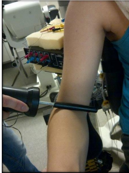
Figure 2.1: Custom-made vibration apparatus. Vibration was applied to the biceps tendon of the less-affected arm. The frequency and amplitude range of the vibration apparatus was 100Hz and 3.5-4.0mm. Vibration was applied throughout the isometric ramp contractions.
