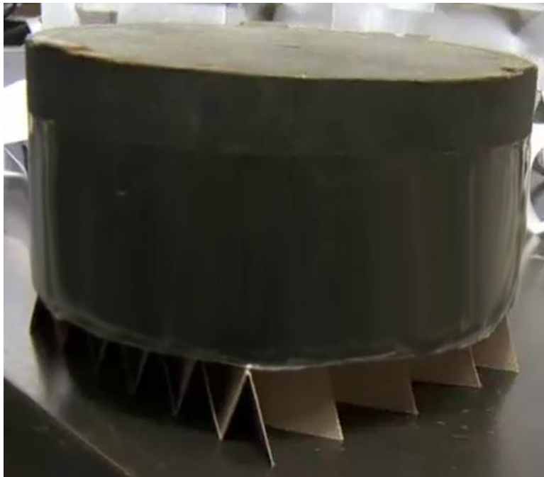
Figure 5.24: High strength paper structure resists a weight of 10 kg.
