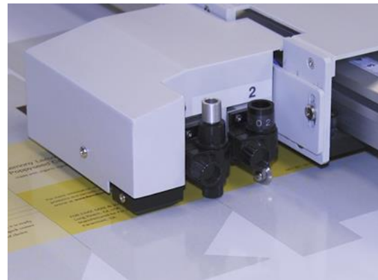
Figure 2.5: Graphtec FC2250-180 dual head design: 500/1000 grams cutting force
