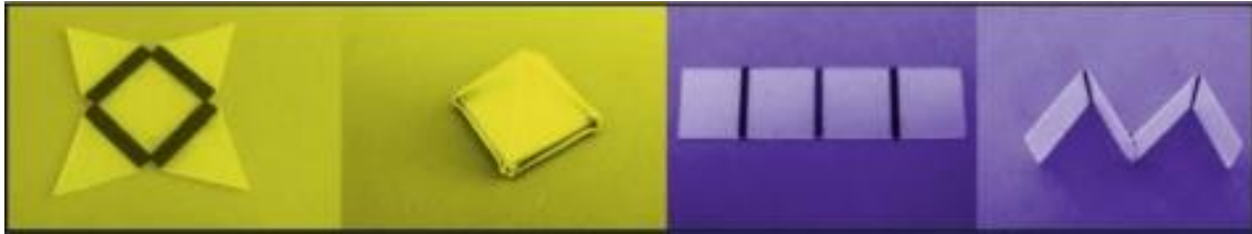
Figure 1.7: 3D structures created by self-folding of Shrinky Dink® patterned with a desktop printer.
