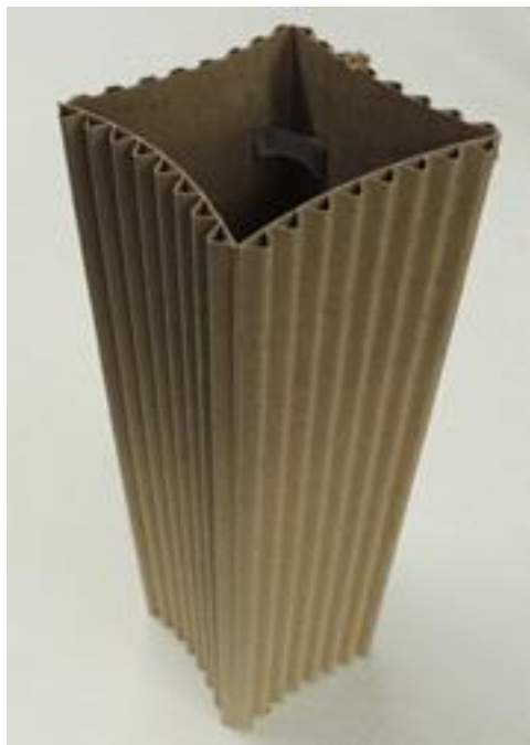
Figure 4.8: Folded linerboard with single faced corrugated board
