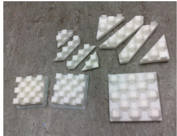
Figure 1.4: Multipart molds with different draft angles
