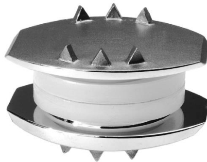
Figure 1-16: Charité artificial disc. It consists of two end plates that are fixed to adjacent vertebral bodies and a core in between them that is domed on both sides, so that to articulate against the concave surfaces of the end plates. Reprinted from [46] with permission from lippincott williams & wilkins.
