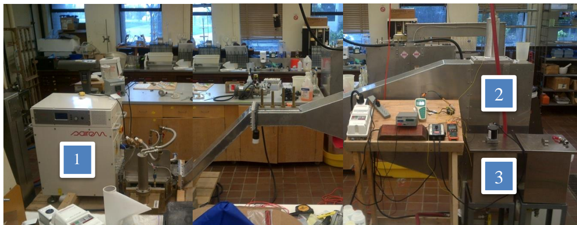
Figure 1: Pilot Scale Microwave System: 1) Generator, 2) Applicator and 3) Reactor System
