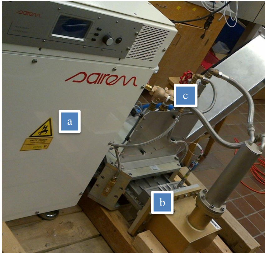
Figure 2: System a) Generator, b) Isolator and c) Water Cooling System
