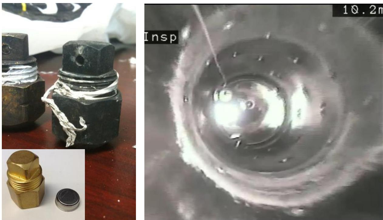
**Figure 3.4** Temperature data logger and chamber (left), and installation set-up at ~10m below ground just above leachate level in an LFG well (right)
