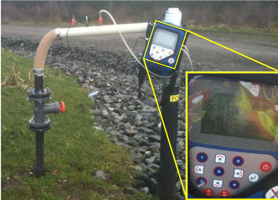
**Figure 3.17** LFG wellhead and LANDTEC GEM2000+ used to collect gas data at VLF
