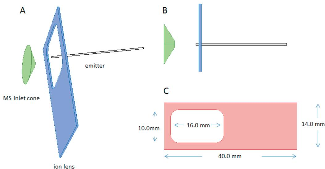
Figure 7.1. Ion Source Setup
