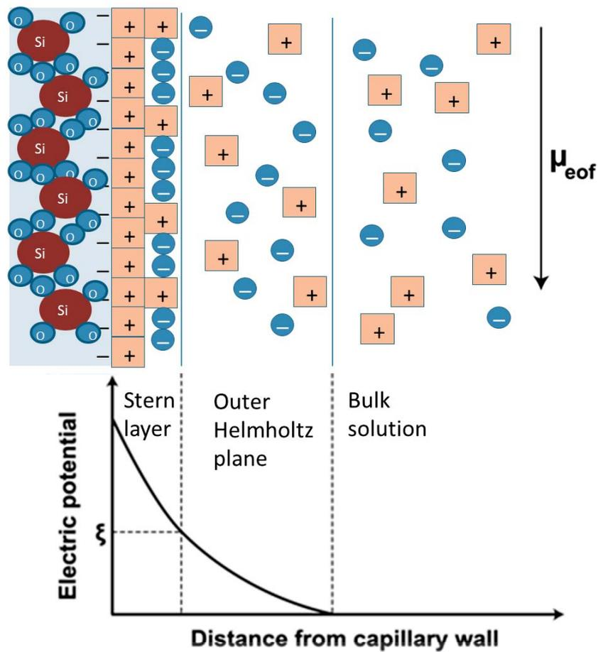
Figure 1.2. Schematic diagram of electrical double layer
