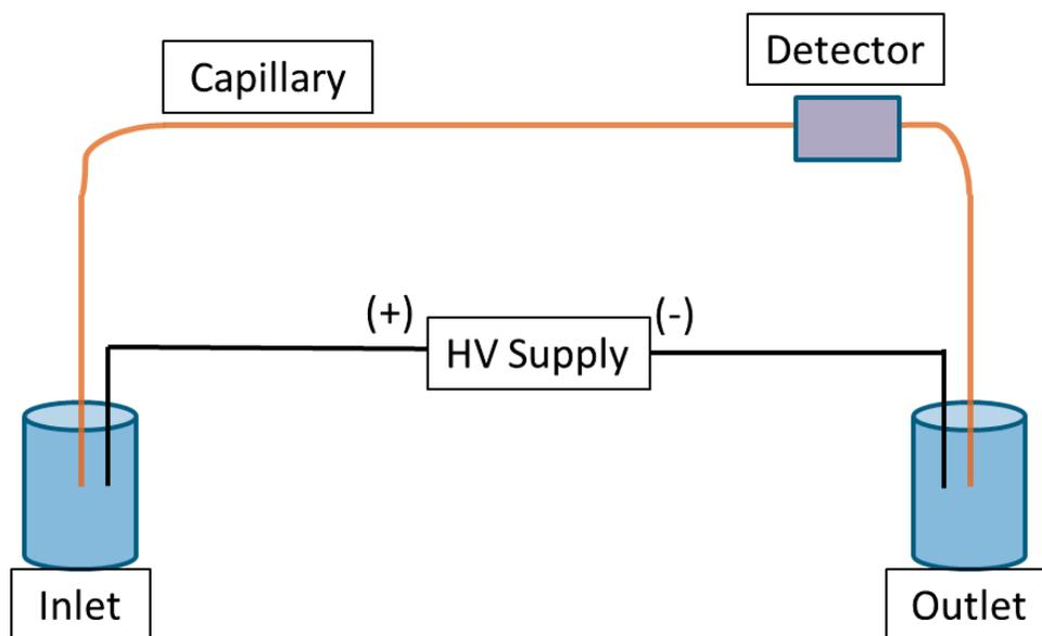
Figure 1.1 CE instrument set-up
