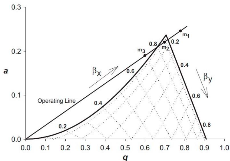
Figure 1.7. The first stability region of quadrupole with an operating line.<sup>61</sup> Reproduced from Elemental analysis with quadrupole mass filters operated in higher stability regions with permission of The Royal Society of Chemistry.
