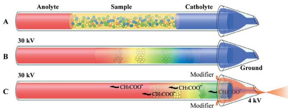
Figure 3.1. Schematic Diagram of Automated cIEF-MS
