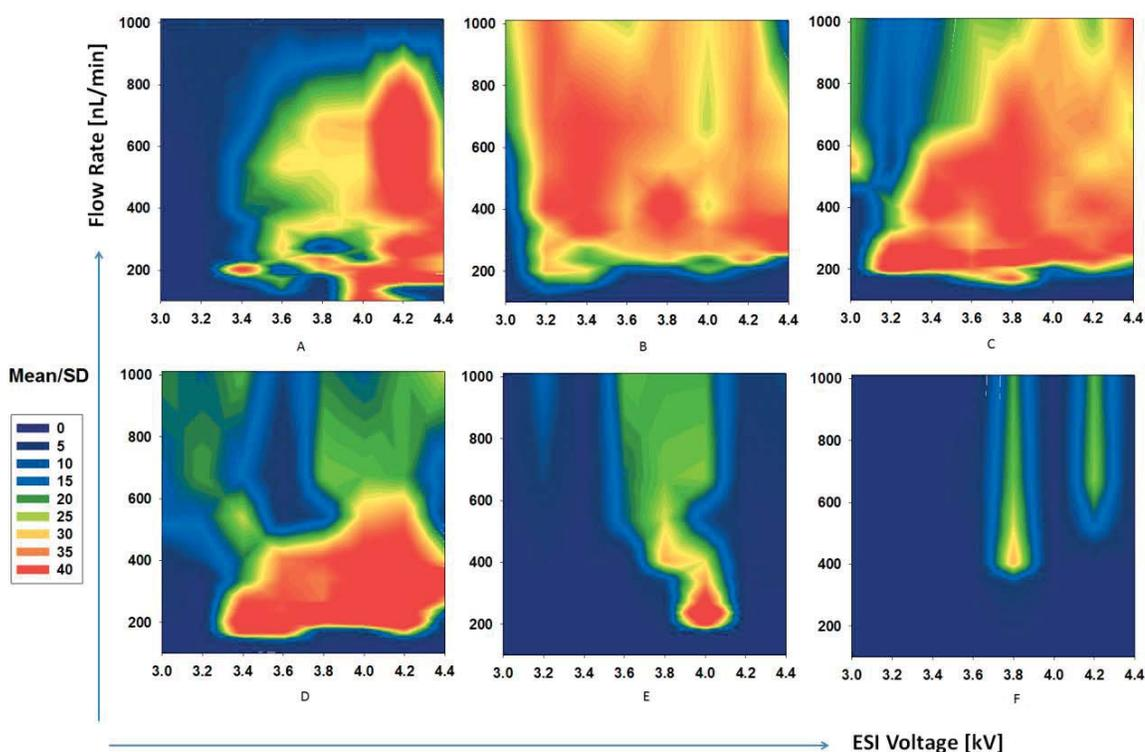
Figure 7.2. Stability Region Comparison under Different Sprayer-Ion Lens Voltage Differences by Pressure Infusion
