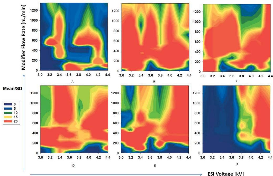
Figure 7.3. Stability Region Comparison under Various Sprayer-Ion Lens Voltage Differences by CE Continuous Infusion with Different Modifier Flow Rates
