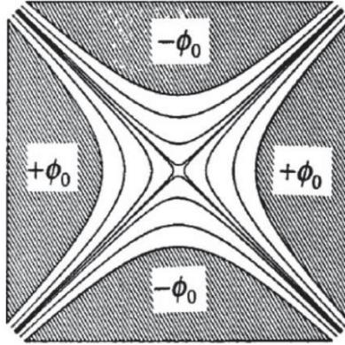
Figure 1.6. Quadrupole with hyperbolic rods and applied potential. Reproduced from Elemental analysis with quadrupole mass filters operated in higher stability regions with permission of The Royal Society of Chemistry.
