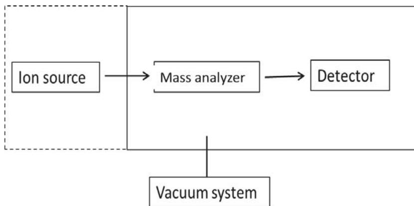
Figure 1.4. General set-up for a mass spectrometer
