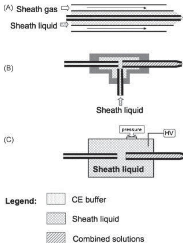
Figure 1.10. Common sheath-flow interface arrangements.
