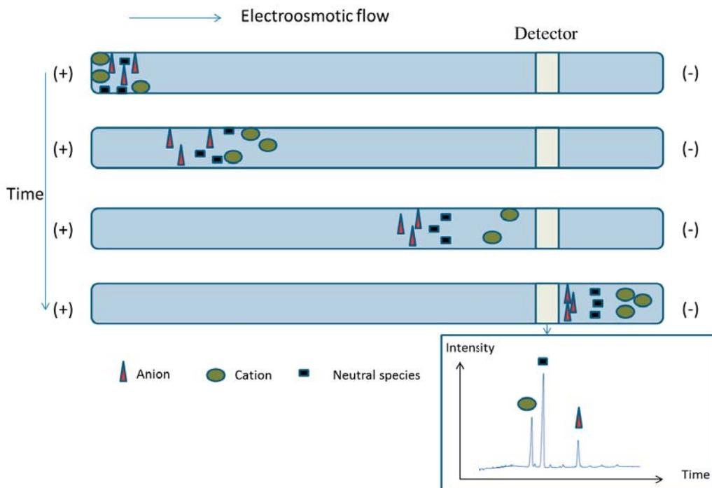
Figure 1.3. Schematic CE separation
