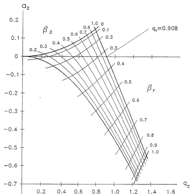
Figure 1.9. A stability diagram of the 3D ion trap
