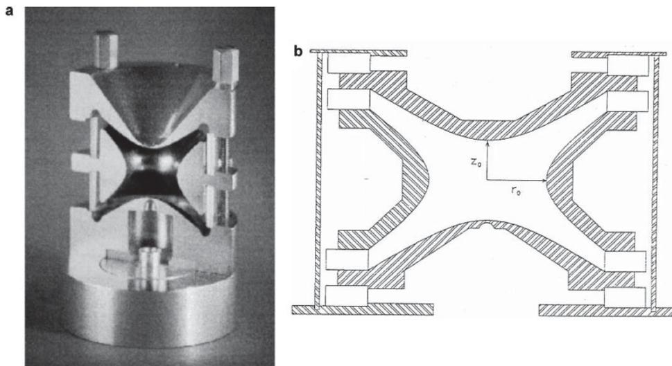
Figure 1.8. A typical 3D ion trap mass analyzer
