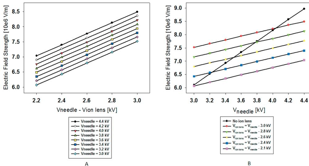
Figure 7.6. Electric Field Strengths as Functions of Sprayer Voltage and Voltage
