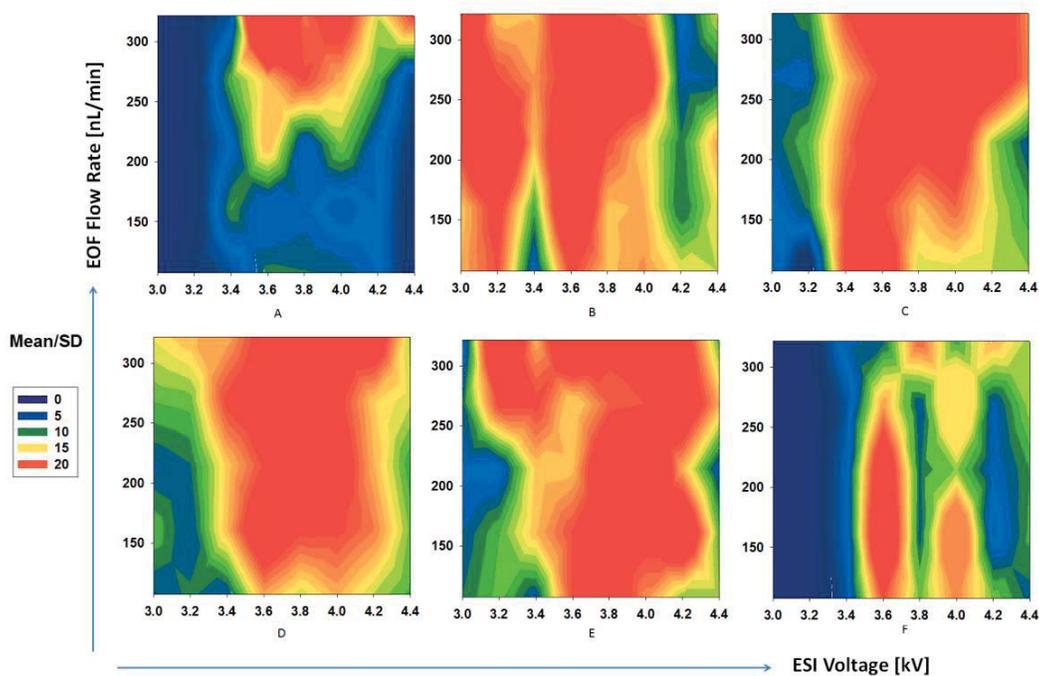
Figure 7.4. Stability Region Comparison under Various Sprayer-Ion Lens Voltage Differences by Different CE Continuous Infusion Flow Rates
