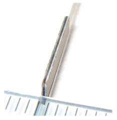
(a) Pizeoceramic plates sandwiching conductive centre shim
