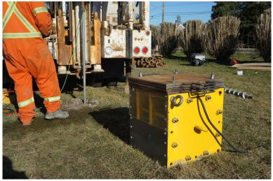
(b) Seismic cone with true interval module
