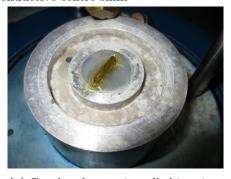
(c) Bender element installed in triaxial end platen
