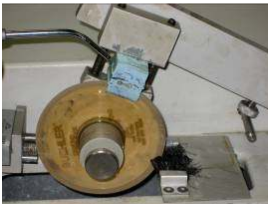
Figure 3-10: Buehler low speed saw sectioning the resin-tooth complex.
