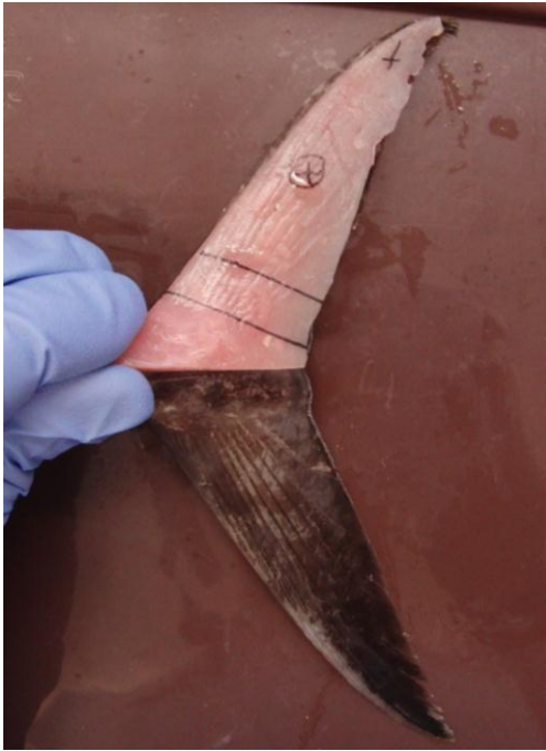
Figure 11- Tail Model: Final model tail made of Flexacryl superimposed on top of the original tail specimen. Parallel lines indicate location of material testing constraints, while the circled cross indicates location of test.
