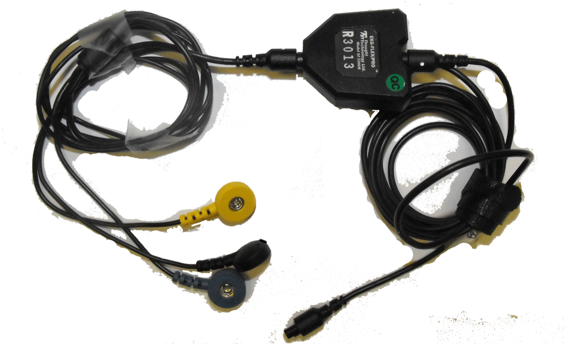
Figure 3.17: Thought Technology EKG™ Sensor T9306M , attached to triode electrodes for placement on chest.
