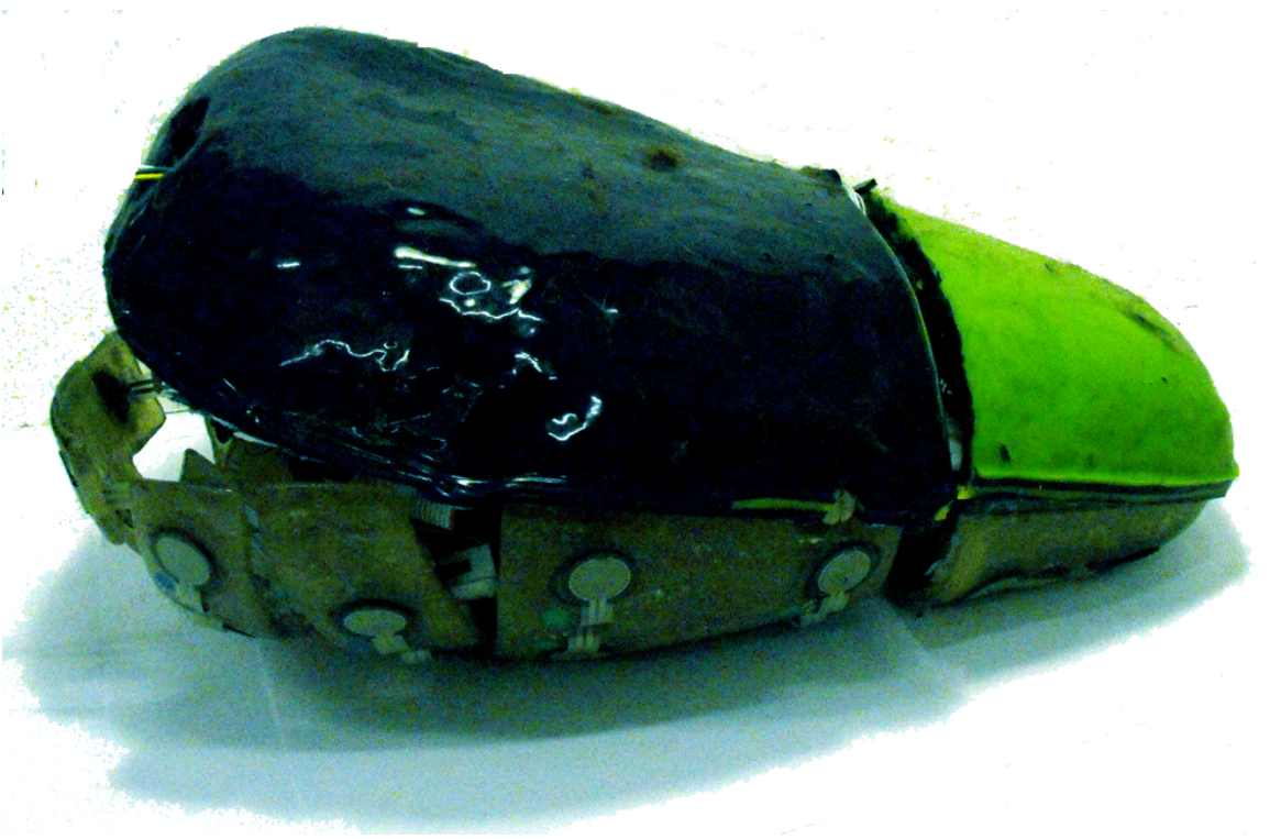
Figure 3.5: The Haptic Creature, upside-down, with fur removed, showing silicone skin.
