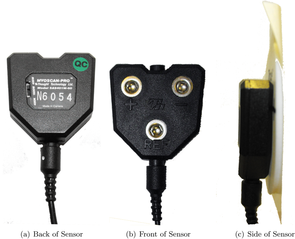
Figure 3.18: Thought Technology EMG MyoScan-Pro™ Sensor T9401M-60 . (c) shows sensor with electrode attached.
