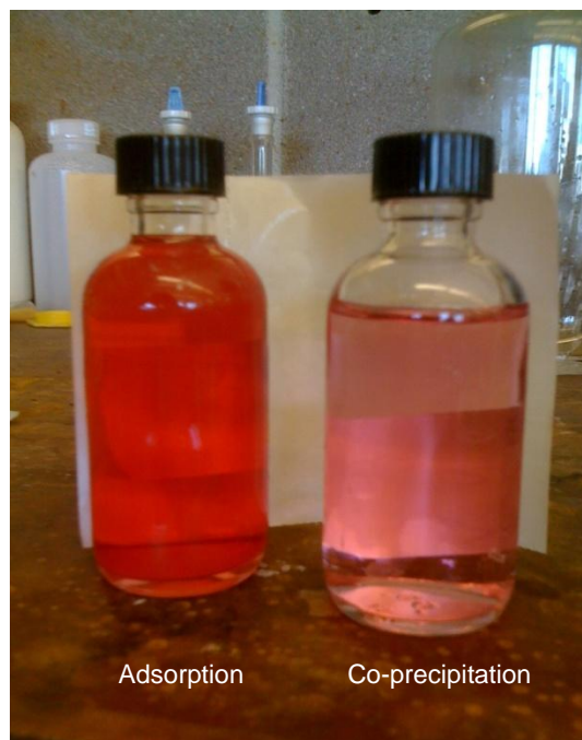
Figure 5.6: The filtrates of the result of adsorption and co-precipitation at 35°C with 0.15 M Fe for 2 hours at pH 7
