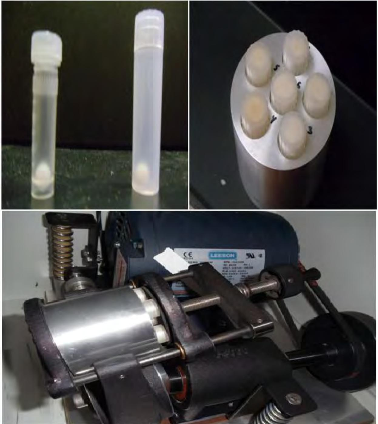
**Illustration C:14 Pulverizing Vials and Aluminum Multiple Sample Holder for 8000M Mill**
