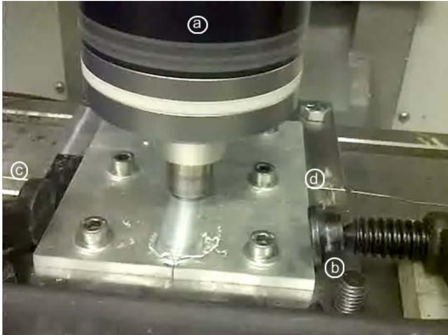
**Figure 9.1-** LowStir™ device (a), FSW test fixture (b) with two embedded thermocouples (c) and (d)
