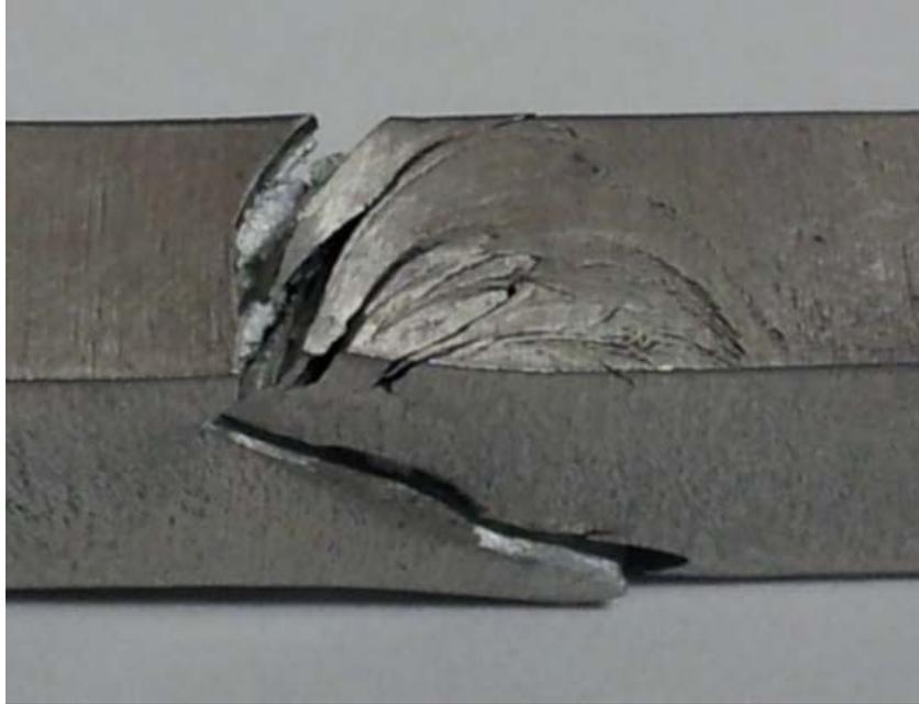
**Figure 9.16-** Fracture zone under the tool pin in sample 7n (cold weld or 1000 RPM, 75 mm/min); notice the delaminated regions in vicinity of the weld line
