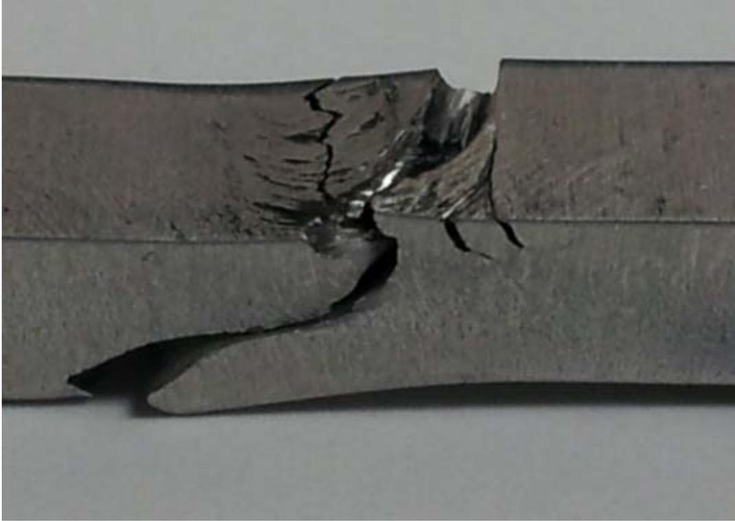
**Figure 9.18-** Fracture zone under the tool pin in sample 3n (hot weld or 1800 RPM, 45 mm/min); notice the delaminated regions in vicinity of the weld line
