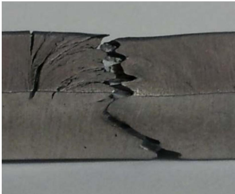
**Figure 9.17-** Fracture zone under the tool pin using sample 2n (1400 RPM, 45 mm/min) with the lowest average axial force; notice the delaminated regions in vicinity of the weld line
