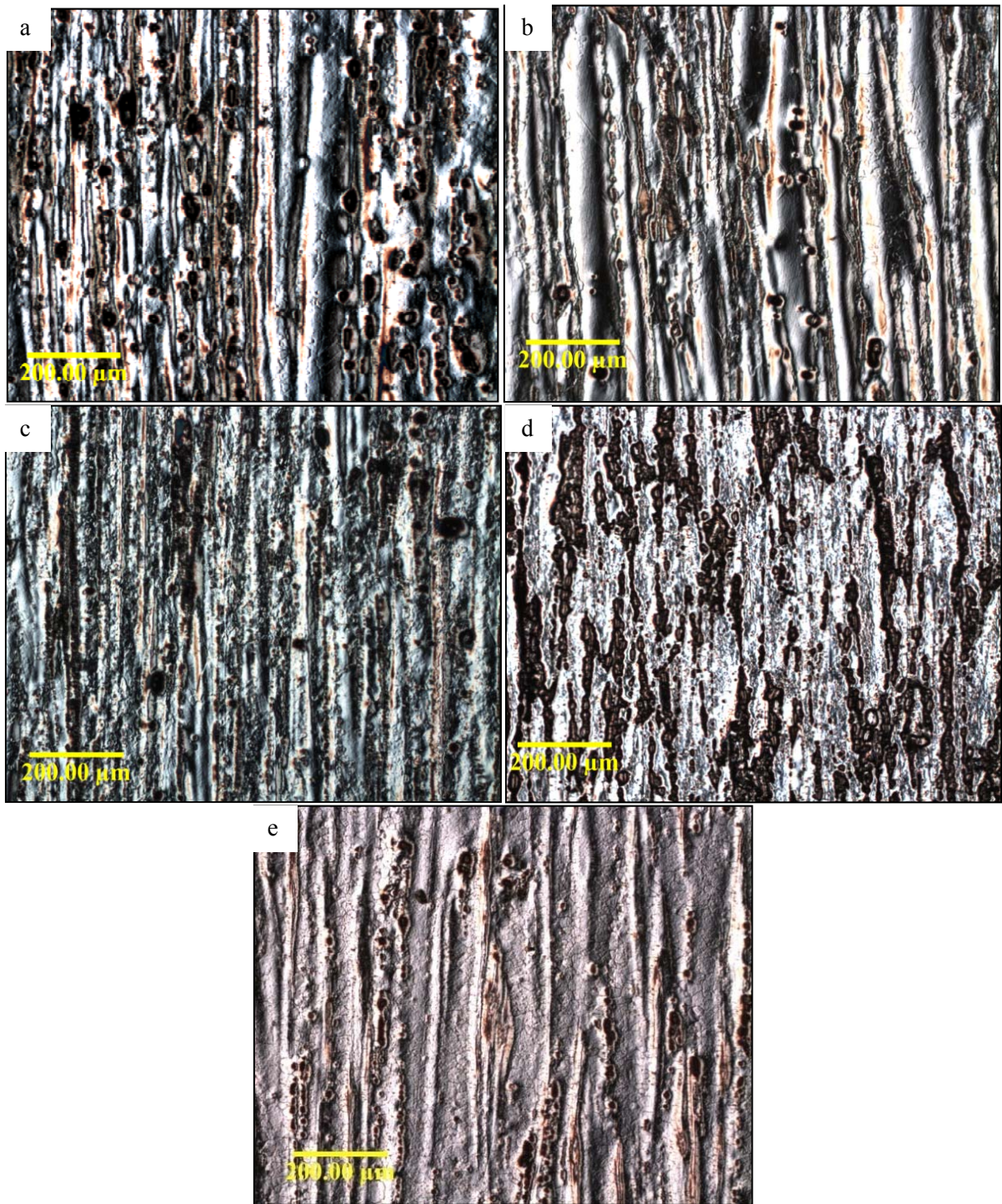
Figure 52. Representative micrographs for the cross-section samples of the: a) AE42 alloy, b) AJ32 alloy, c) AX30 alloy, d) EZ33 alloy and e) ZE10 alloy
