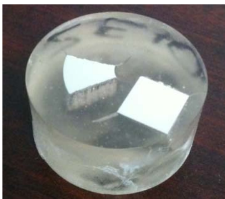
Figure 30. Representative example of the mounted and polished sample
