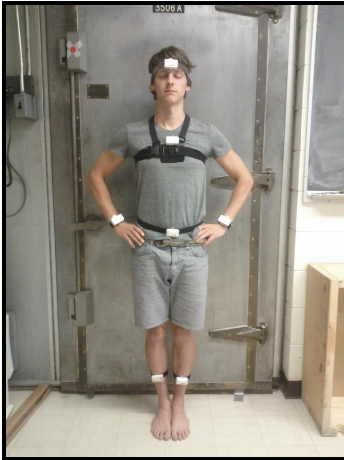
Figure 4.1. Subject performing the two-foot firm surface balance condition of the Balance Error Scoring System (BESS) while wearing inertial measurement units (IMUs) secured to seven landmarks of the body: forehead, sternum, waist, right & left wrist, and right & left shin.
