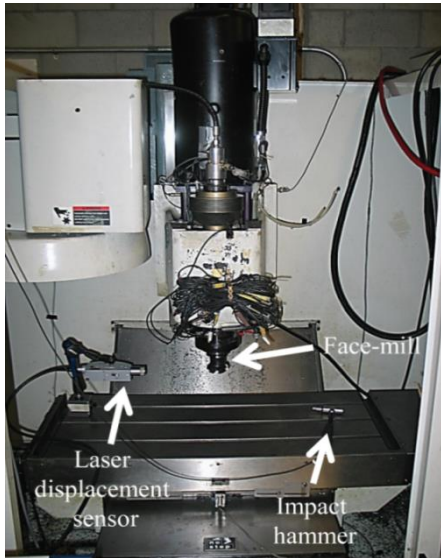
Figure 5.5 Experimental setup to measure TCP FRFs on machine.
