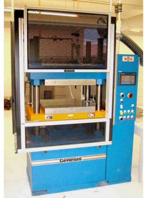
Figure 4-2 (a) Forming cycle used for preparing PPS/Glass test samples using (b) an automated press apparatus (Wabash MPI 100 ton)
