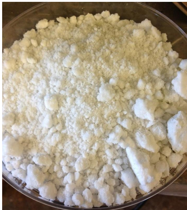
FIGURE 4.7 CRYSTALLINE PRECIPITATE #2 SYNTHESIZED BY ADDITION OF SOLID SODIUM SULFIDE TO SODIUM ARSENATE SOLUTION
