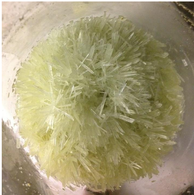
FIGURE 4.10 CRYSTALLINE PRECIPITATE #4 SYNTHESIZED BY REACTION OF ELEMENTAL SULFUR (12.8 G) WITH ARSENIC TRISULFIDE (50 G) IN 200 ML AT 3M SODIUM SULFIDE
