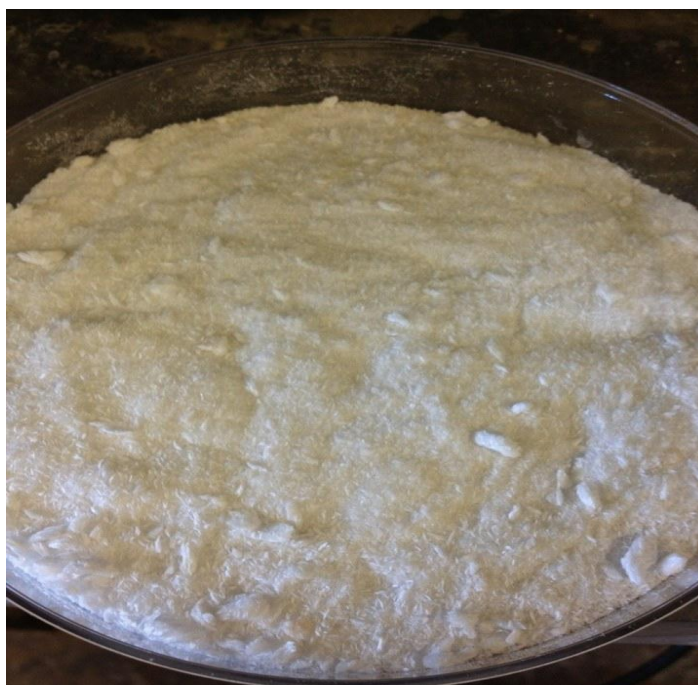
FIGURE 4.6 CRYSTALLINE PRECIPITATE #1 SYNTHESIZED BY ADDITION OF SODIUM SULFIDE SOLUTION TO SODIUM ARSENATE SOLUTION
