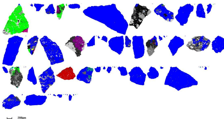
Figure 4.3.1.3. Typical particle line-up of false-colour segmented particles (FC-2, -1190/+600 µm, mosaic frame-merge).
