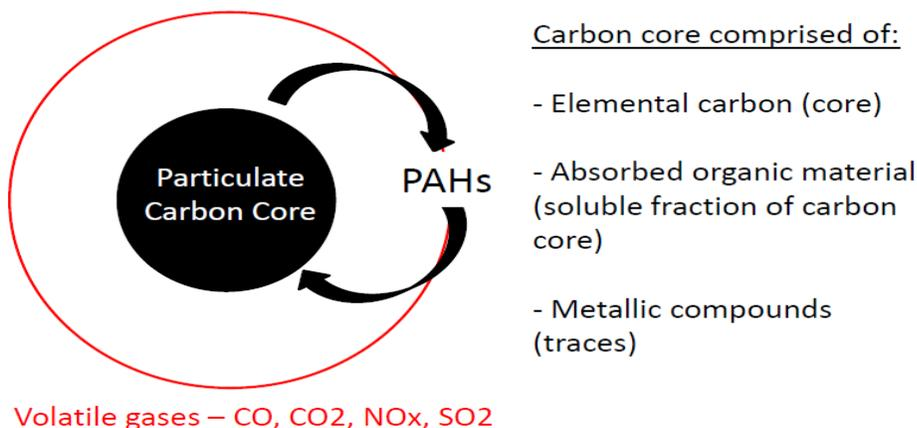
**Figure 1. Diesel engine exhaust chemical structure substitute.** Absorbed organic material refers to the PAHs which dissolve and get emitted by the carbon core depending on the ambient environment. Metallic compounds include lead, arsenic, etc, which are highly toxic materials. Depending on the type of diesel fuel, there may or may not be sulfur and sulfur oxides being emitted.
