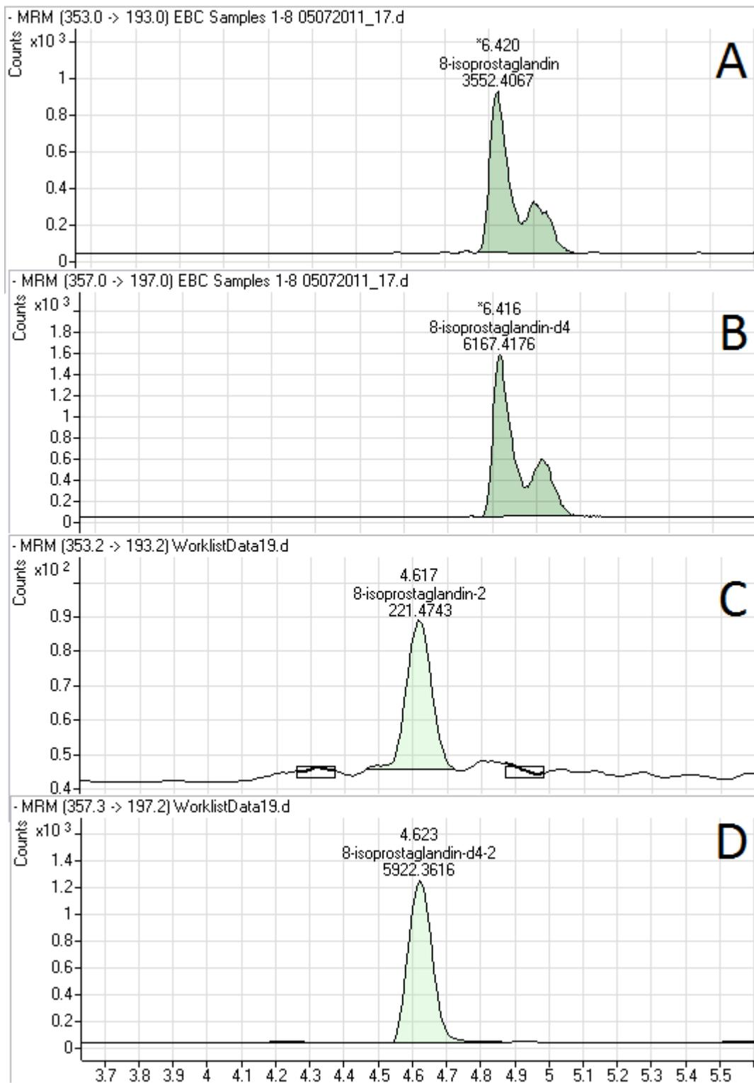
**Figure 15.** LC-MS/MS chromatogram of an exhaled breath condensate sample spiked with A) 1011.6 pg/ml standard solution of 8-iso-PGF2 $\alpha$ , B) 2012.3 pg/ml internal standard 8-iso-PGF2 $\alpha$ -d4, using the pre-optimized method. LC-MS/MS chromatogram of an exhaled breath condensate sample spiked with C) 744.5 pg/ml standard solution of 8-iso-PGF2 $\alpha$ , D) internal standard 8-iso-
