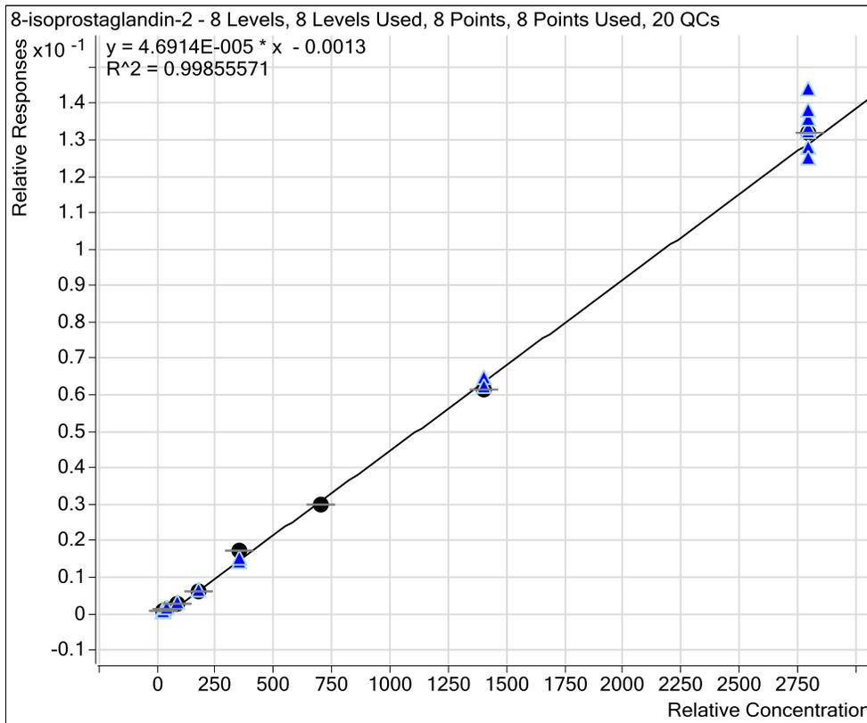
**Figure 14. Calibration curve for present method.**
