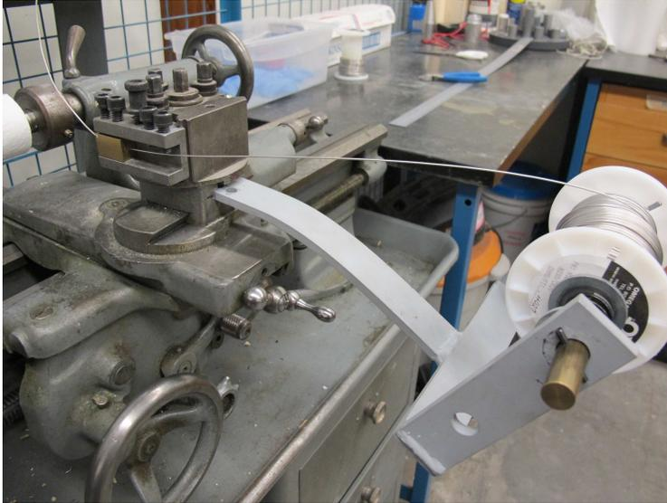
**Figure C 7: Spool holder in lathe and wire loaded into wire feed.**
