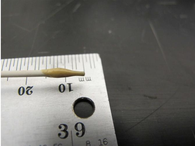
**Figure C 16: Ceramic coating on thermocouple to avoid short circuiting**
