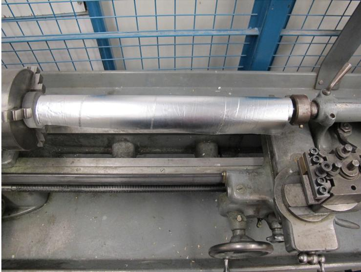
**Figure C 2: Mold wrapped in aluminium foil**
