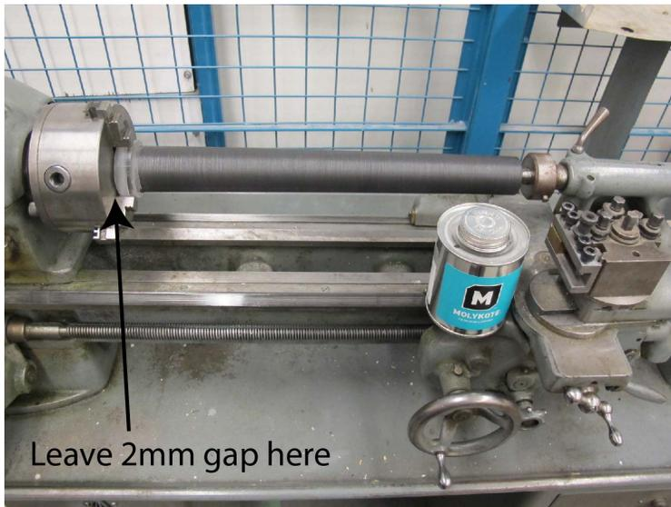
**Figure C 1: Plexiglass mold in lathe, coated in P37 anti-seize paste**
