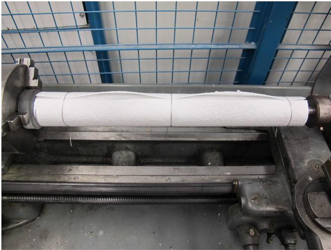
**Figure C 4: Mold wrapped in ceramic paper with tourniquets applied**
