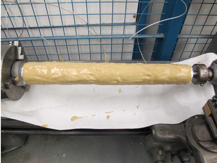
**Figure C 19: Finished heating element drying on mold**
