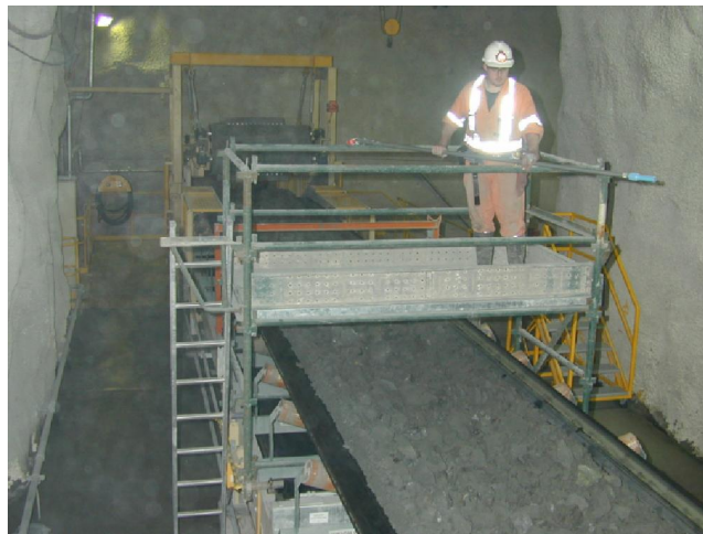
Figure 30: Marker recovery from the collection conveyor belt
