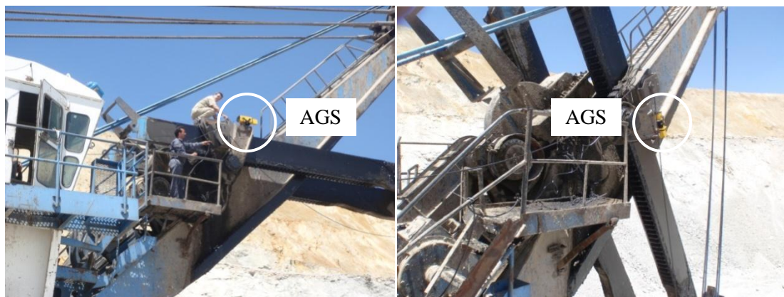
Figure 23: Dipper and AGS positions at two different dipper handle angles
