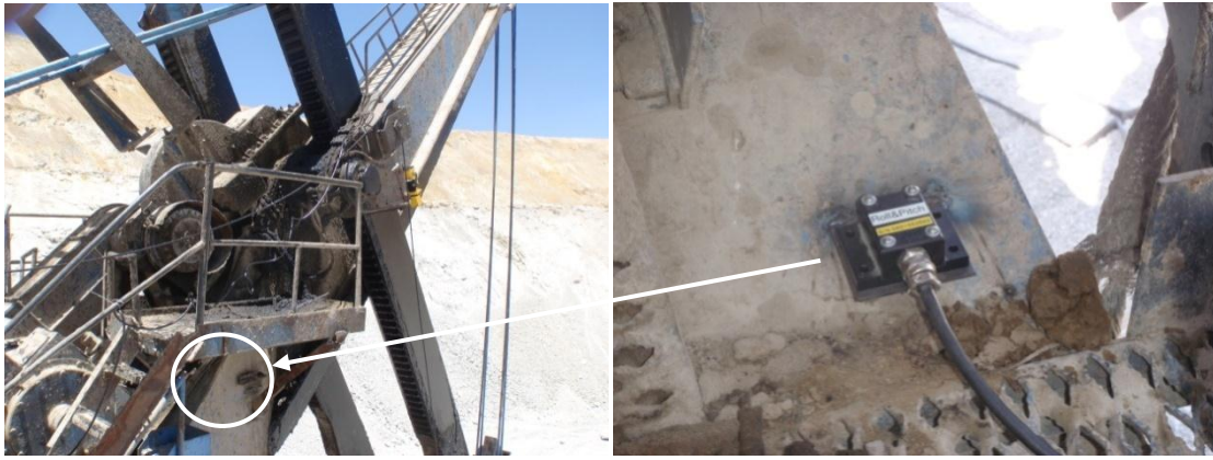
Figure 29: The boom angle sensor installed on the cable shovel boom
