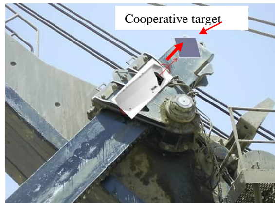
Figure 21: Installation of a cooperative target on the dipper handle
