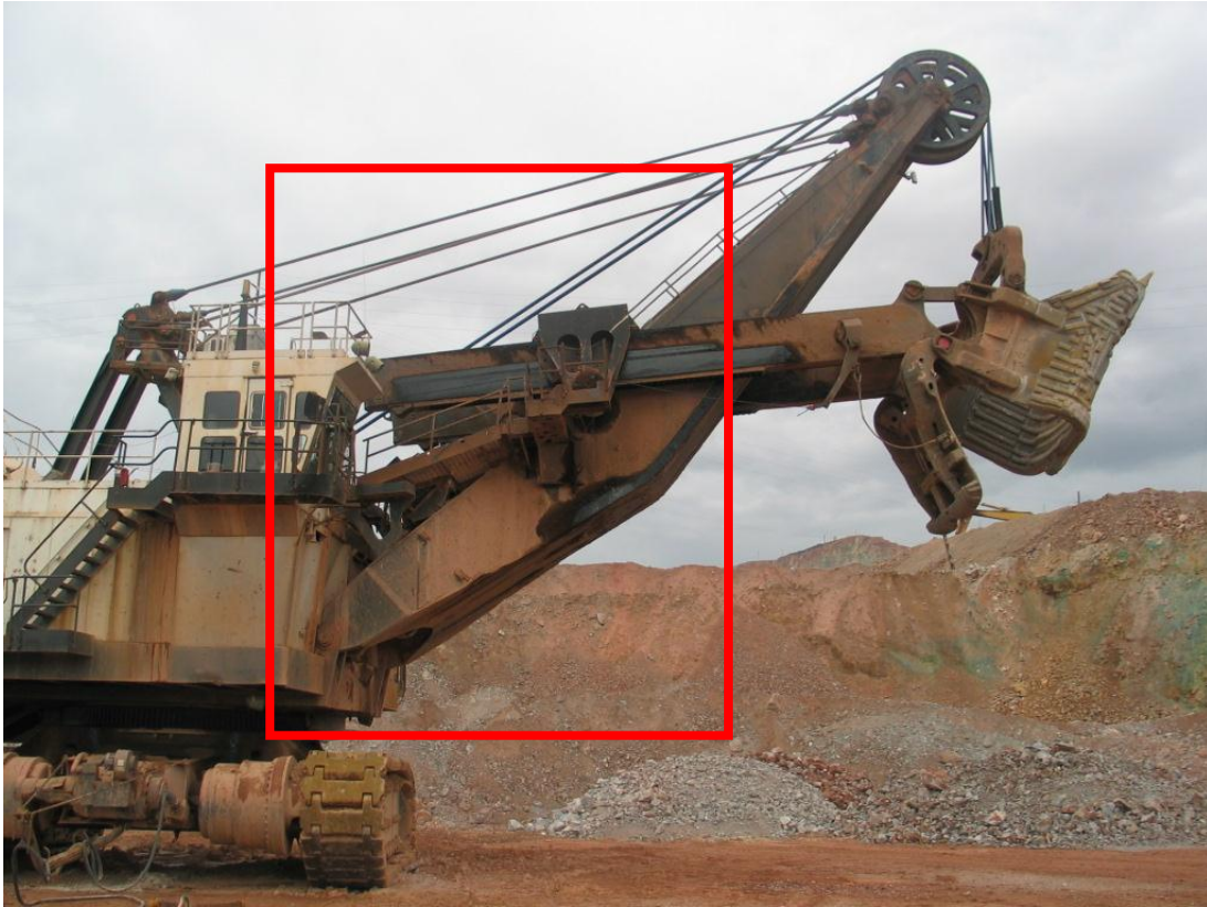
Figure 12: A suitable area for the installation of the arm-geometry sensor.
