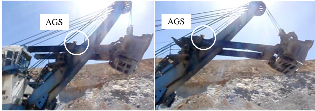
Figure 25: Dipper and AGS positions for two different crowd extension lengths
