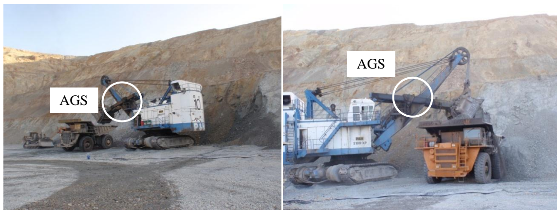
Figure 24: Shovel machinery and AGS positions at two different swing angles
