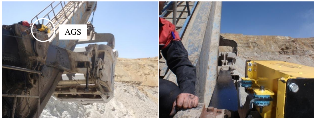
Figure 22: The arm geometry sensor apparatus (AGS) installed on a P&H cable shovel saddle block
