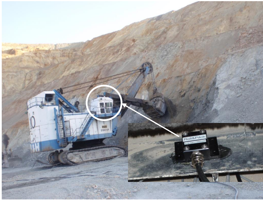
Figure 30: The cab roll/pitch angel sensor installed in the operator cabin
