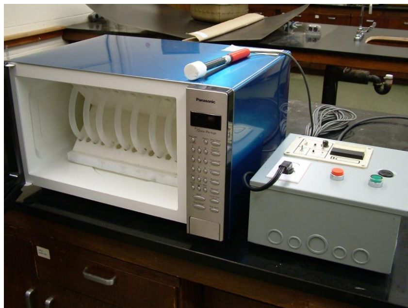
Figure 4.2 Front view of the microwave flow through cell and control box
