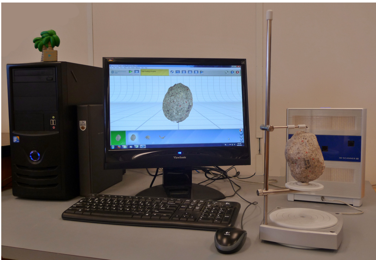
Figure 5-12. NextEngine™ 3-D laser scanner workstation. A personal computer and monitor are connected via USB to the NextEngine™ 3-D scanner (back right). The scanner connects to the AutoDrive sample platform (front right) upon which the sample is positioned, held in place by a movable part gripper.
