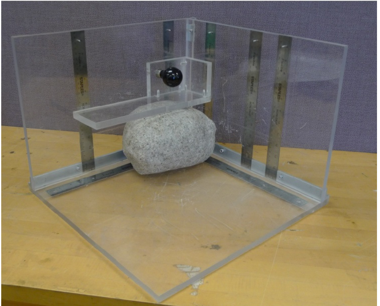
Figure D1-1. Photograph of axis measurement frame used in this study (3-sided plexiglass box, with inlaid rulers).
