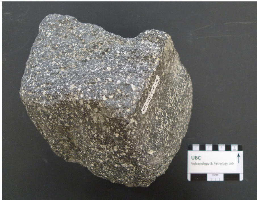
Figure 4-15. Columnar joint surfaces on a dacite accessory lithic clast (Plinth Assemblage). The lower and right faces of the photographed clast are relatively smooth and planar columnar joint surfaces, while the uppermost face is a relatively rough fractured surface.
