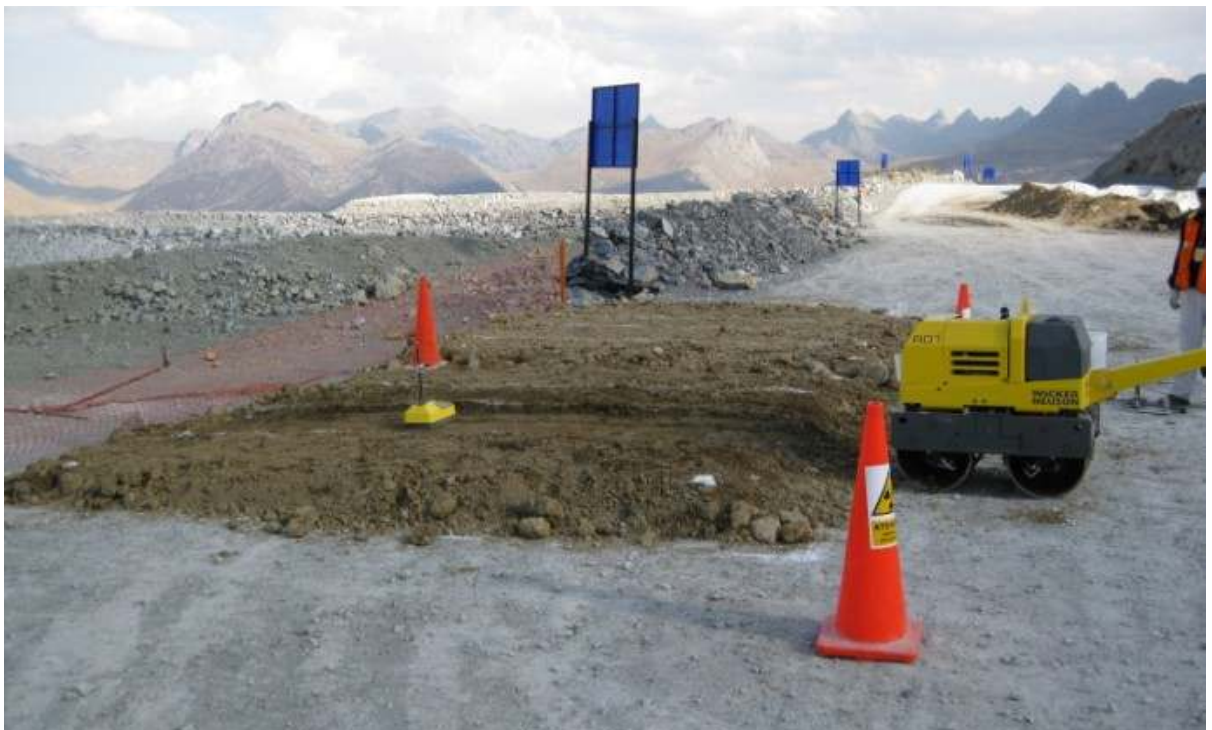
Photo #40: Performing nuclear density test on compaction platform.
