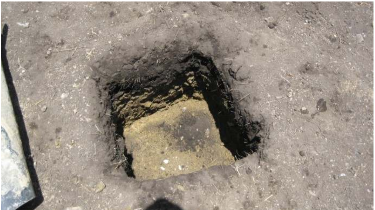
Photo #73: Test pit for installing TC sensors in lysimeter #2.
