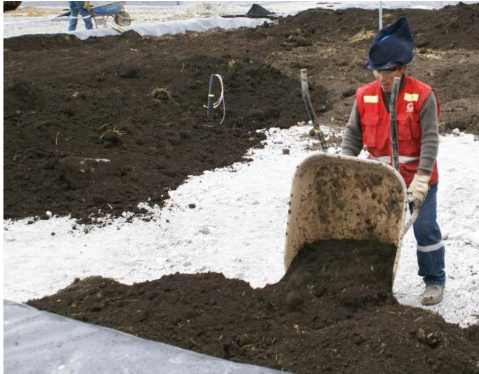
Photo #34: Topsoil cover already placed in lysimeter #4. Oxygen sampling tubes coming out of the cover in the middle of the lysimeter. Standing pipe next to oxygen sampling tubes for Net Radiometer.
