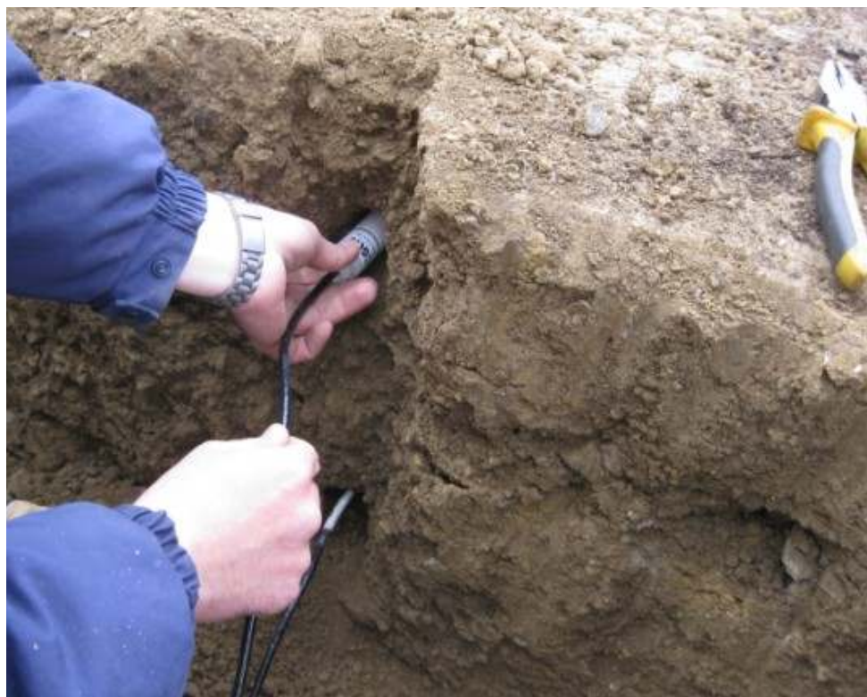
Photo #67: Installing TC sensor in hole left by PVC pipe.
