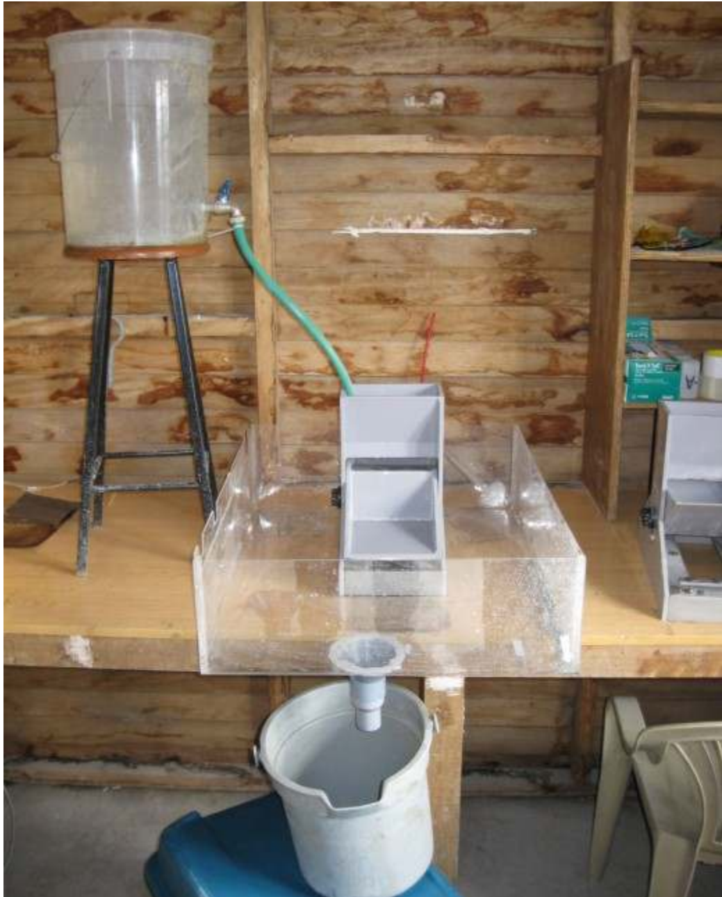
Photo #60: Calibration of tipping buckets.
