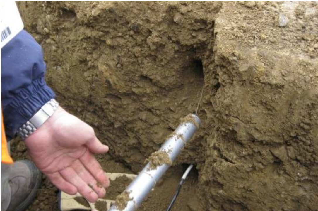
Photo #67: Installing TC sensor in hole left by PVC pipe.
