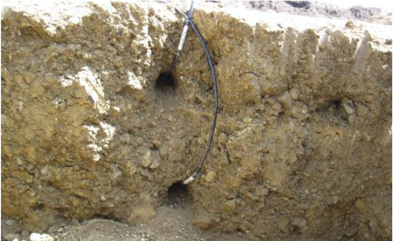
Photo #71: Holes filled with clayey till and expandable foam, with TC sensors inside.
