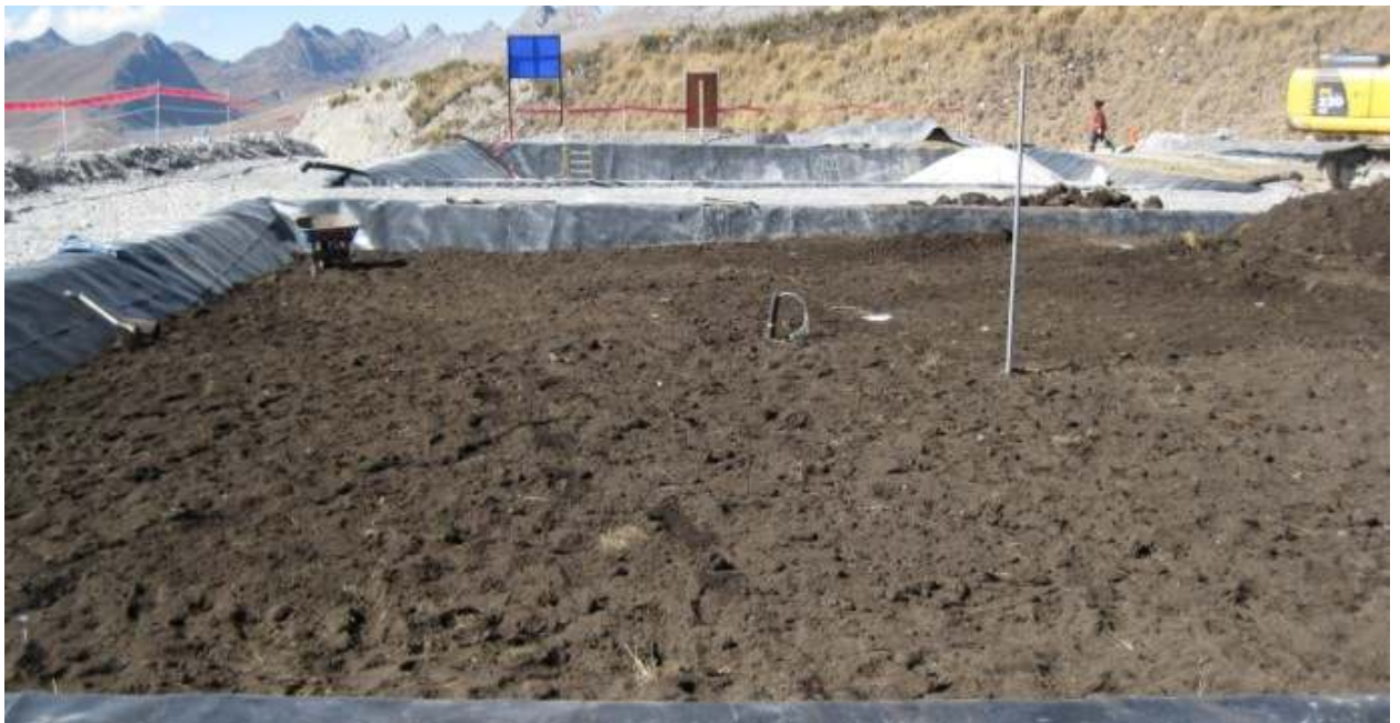
Photo #34: Topsoil cover already placed in lysimeter #4. Oxygen sampling tubes coming out of the cover in the middle of the lysimeter. Standing pipe next to oxygen sampling tubes for Net Radiometer.
