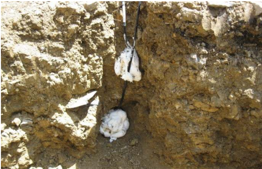
Photo #71: Holes filled with clayey till and expandable foam, with TC sensors inside.
