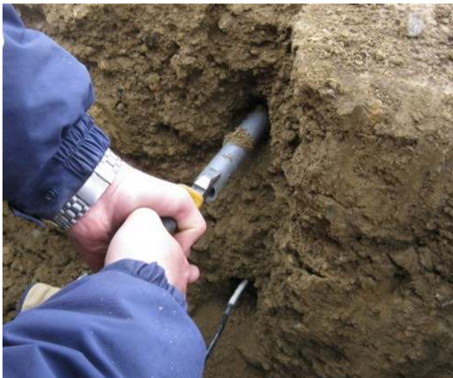
Photo #65: Pulling PVC pipes out of the cover.
