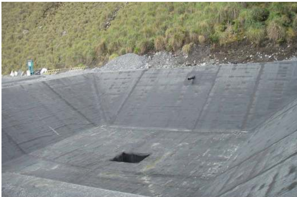
Photo #12: Lysimeter #2 with bituminous liner and run-off and infiltration piping systems already installed.
