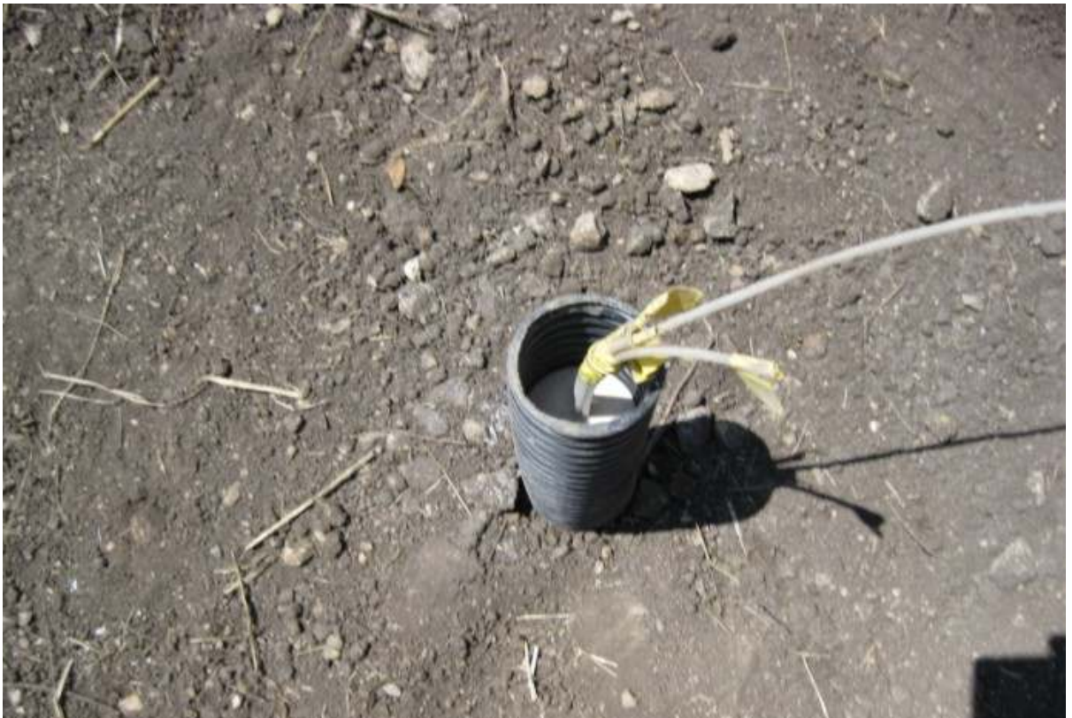
Photo #85: Oxygen sampling tubes coming out of the cover system through HDPE pipe.
