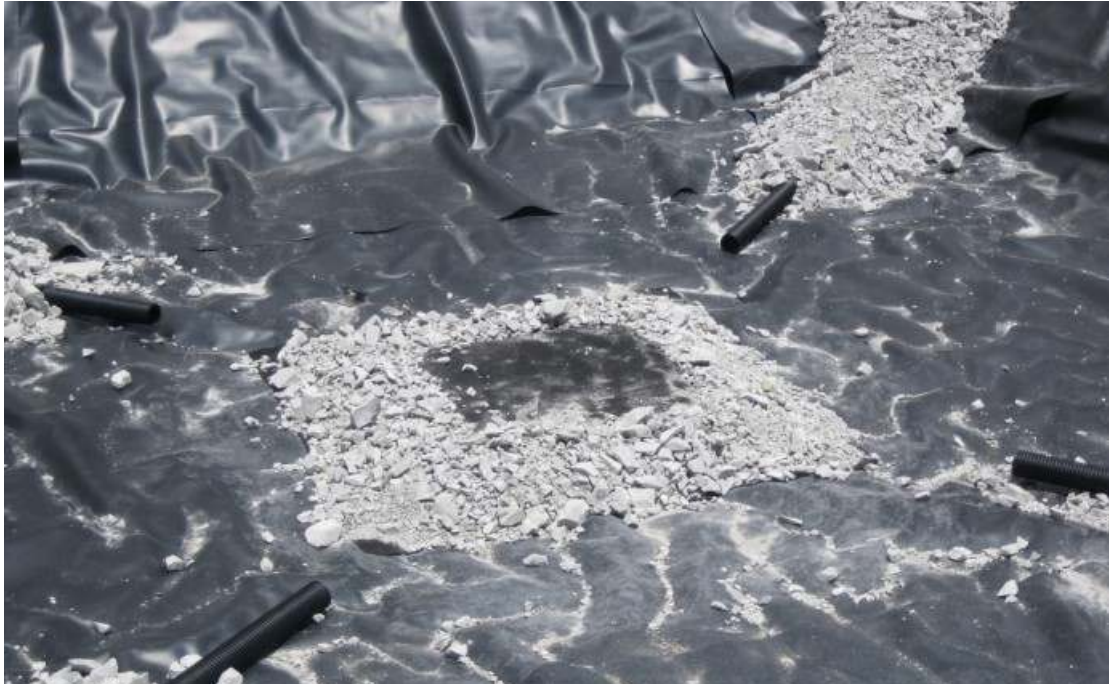
Photo #22: Placing Class A Intrusive in lysimeter #5.
