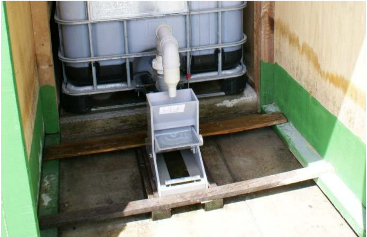
Photo #58: Plastic base for tipping buckets.
