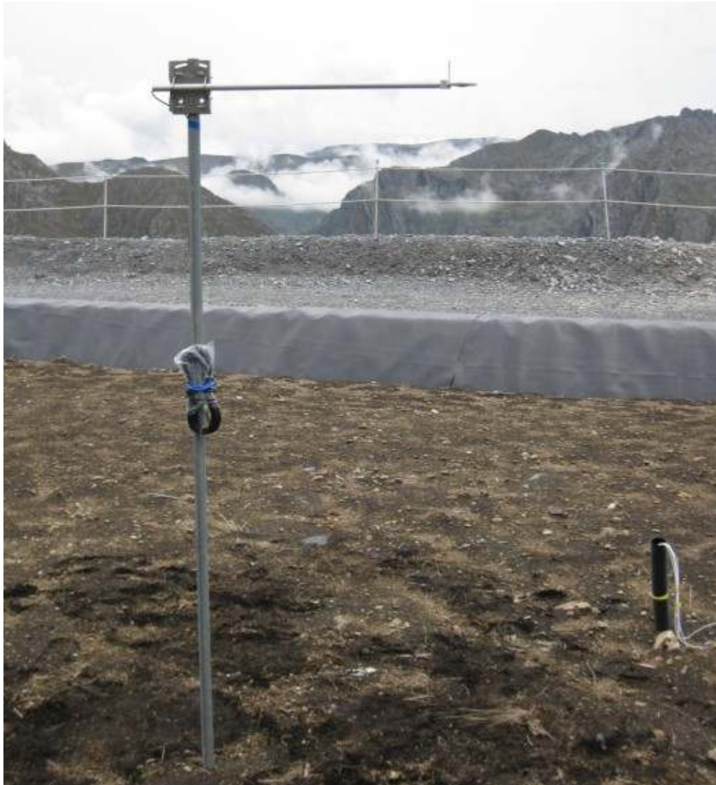
Photo #86: Net Radiometer installed in Lysimeter #4.
