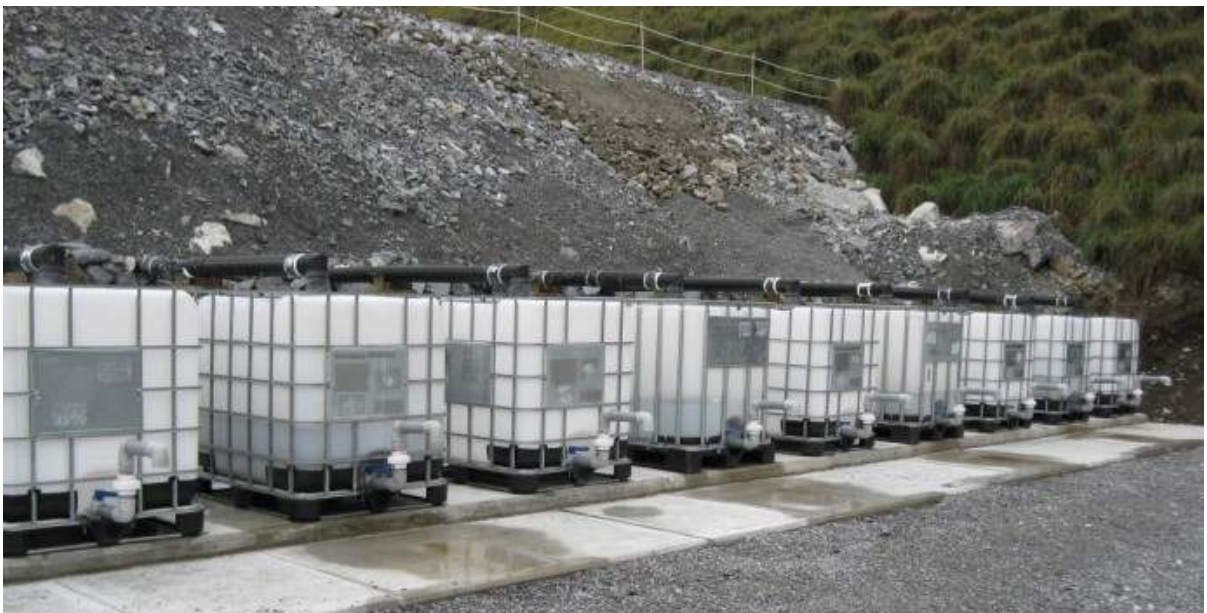
Photo #54: Tanks for collecting infiltration and runoff water.
