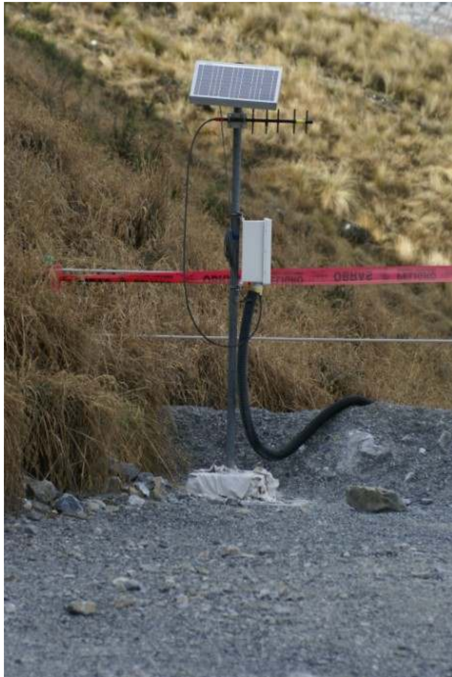
Photo #61: Data logger station for tipping buckets and net radiometer.
