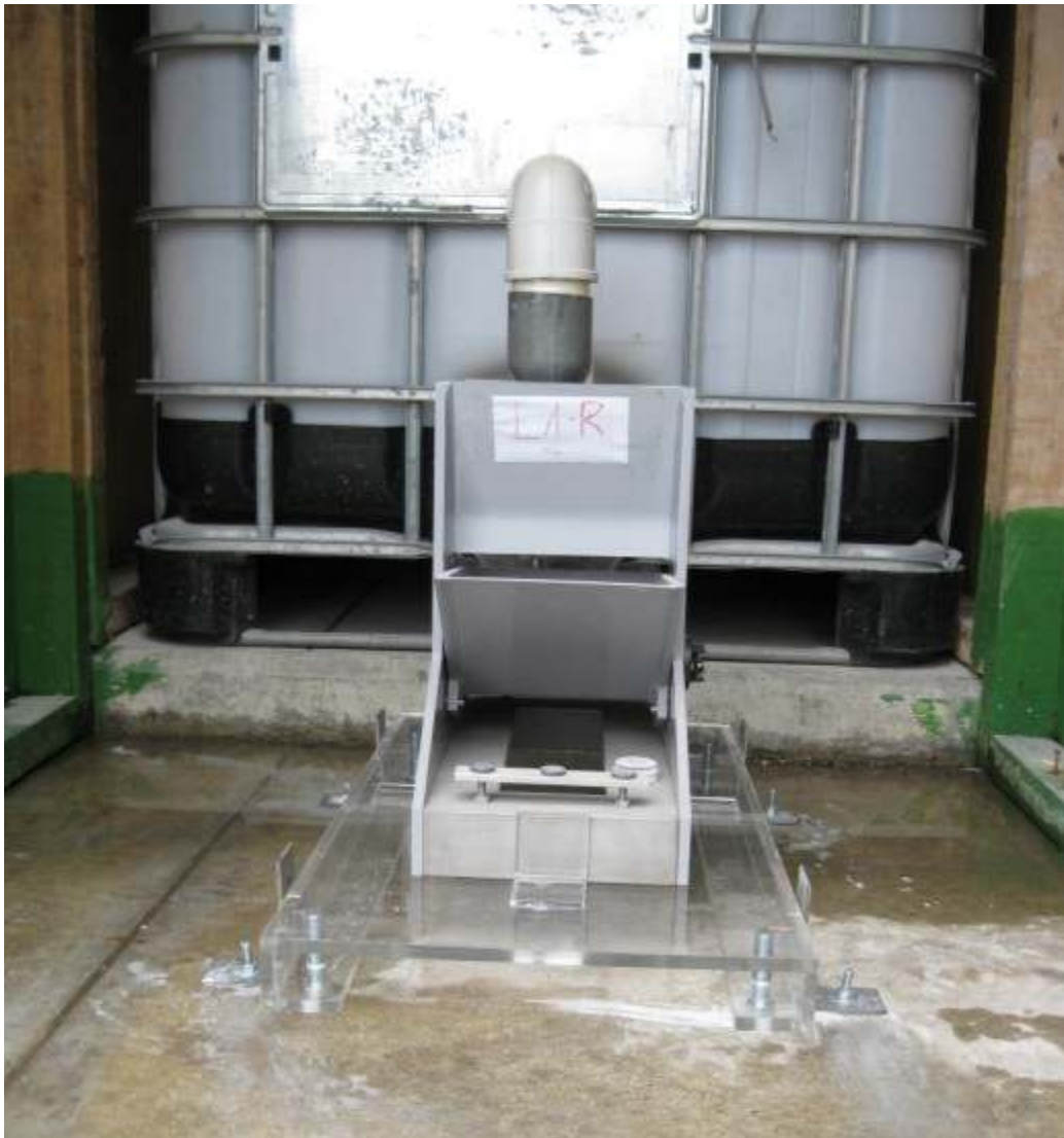
Photo #59: Tipping bucket placed on plastic base.
