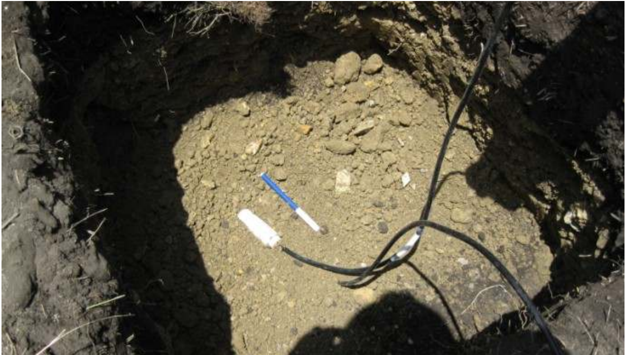
Photo #75: Installing TC sensors in lysimeter #2.
