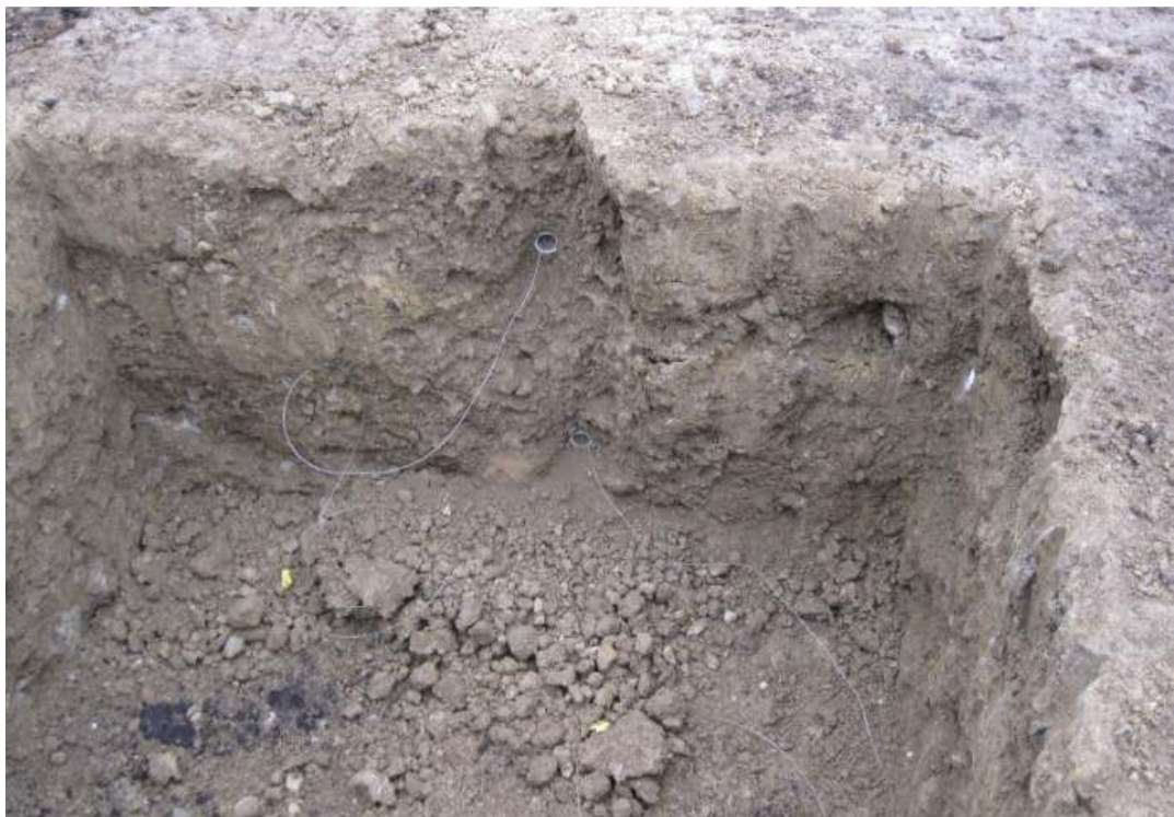
Photo #63: Horizontal PVC pipes left in the cover system to get a hole for TC sensors.
