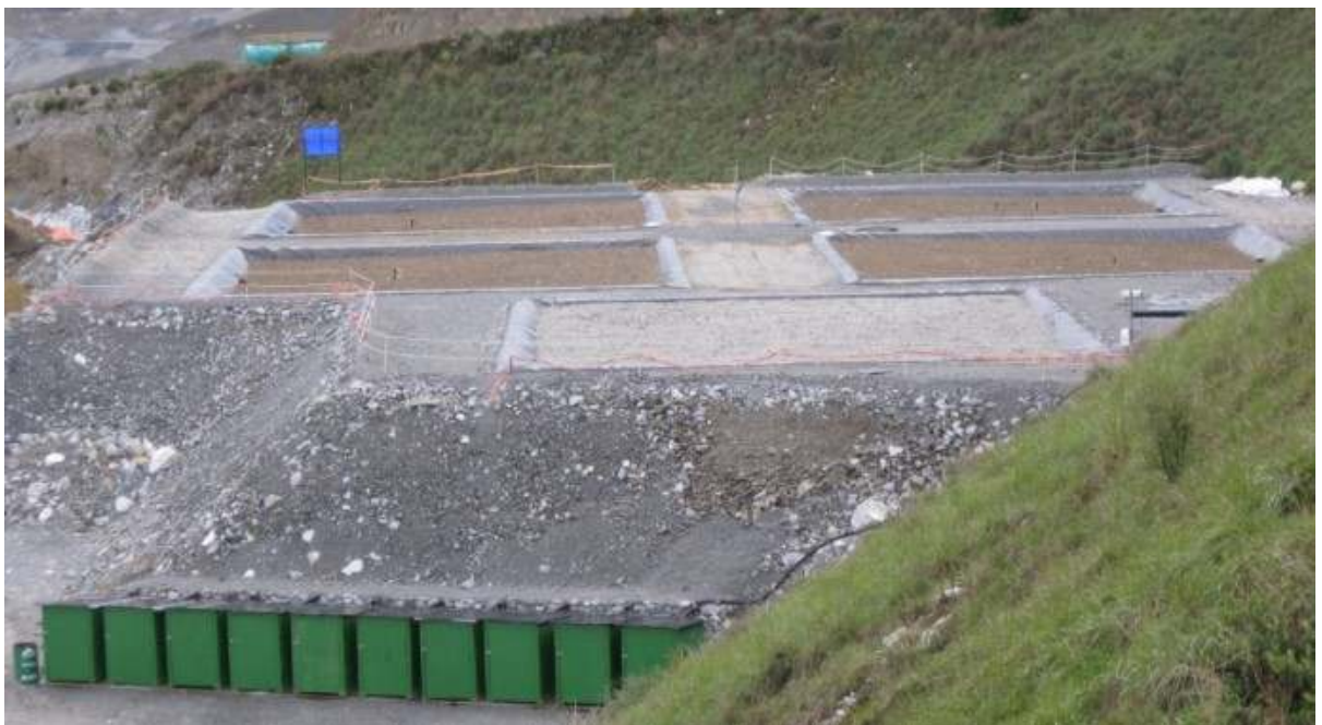
Photo #48: View of the five cover systems already built in the lysimeters.
