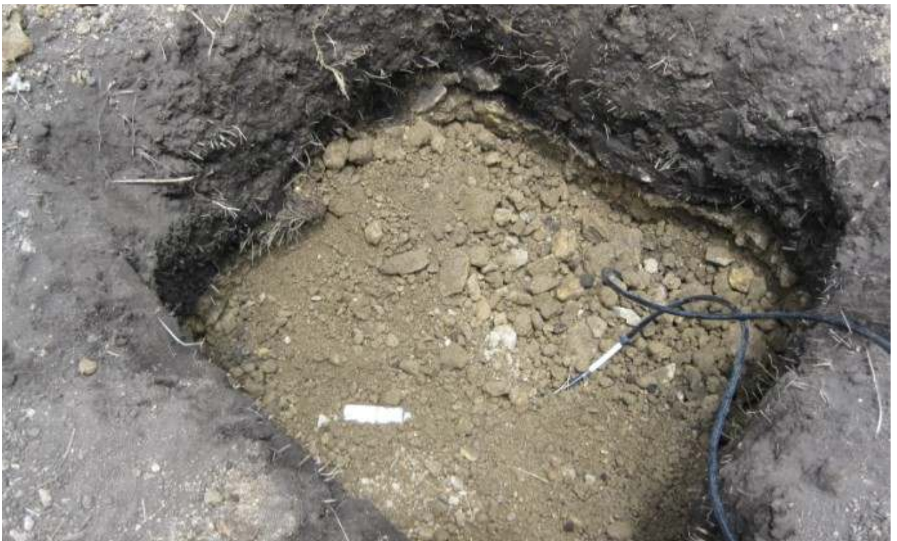
Photo #75: Installing TC sensors in lysimeter #2.
