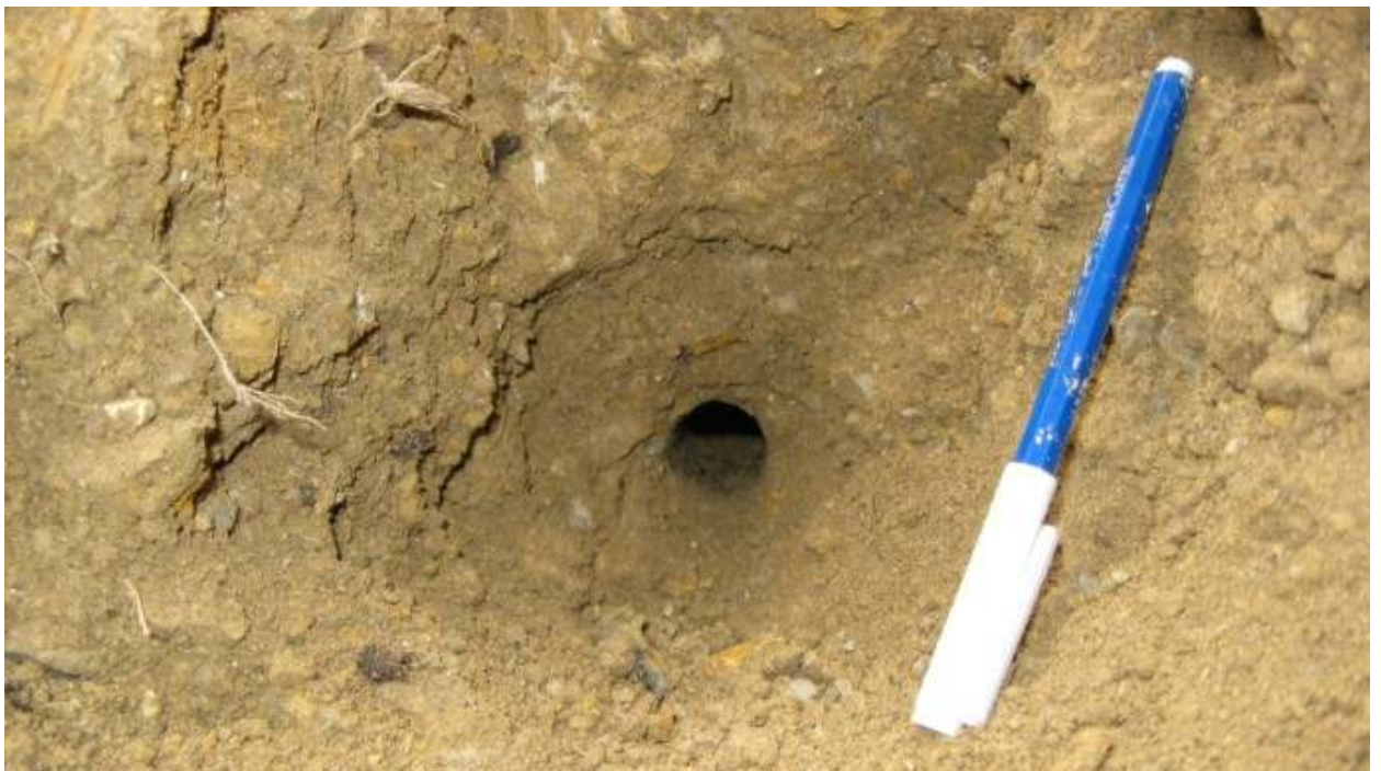
Photo #69: Hole left in silty till cover by PVC pipe.
