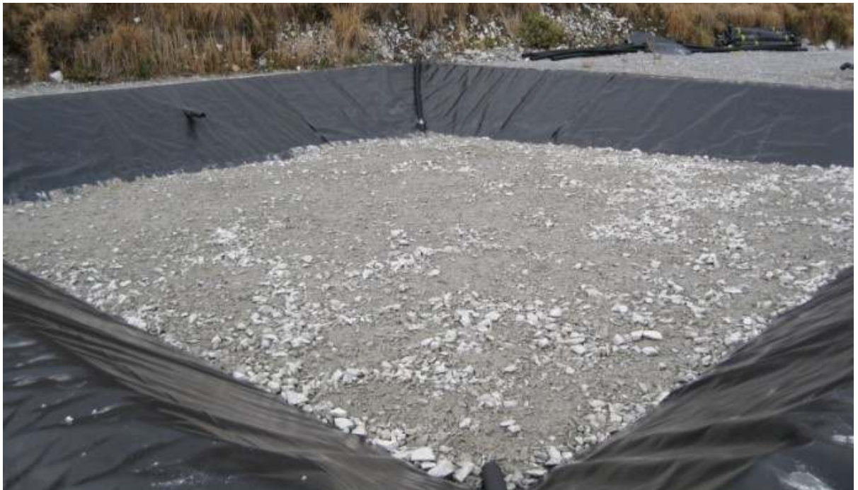
Photo #26: Class A Intrusive already leveled in lysimeter #2.
