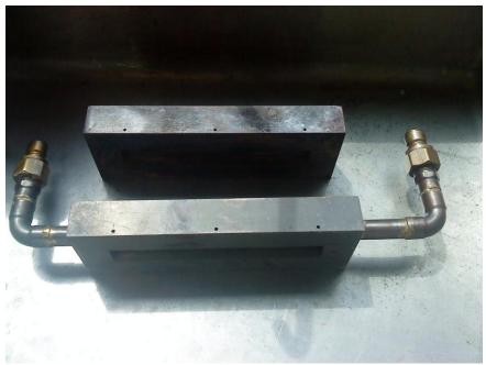
Figure 4.3: The water-cooled and solid chills
