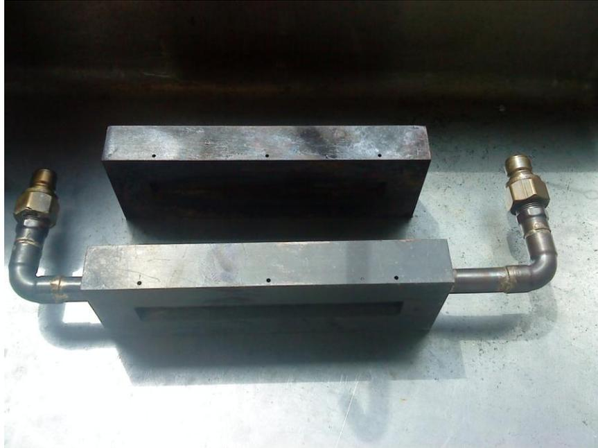
Figure 4.3: The water-cooled and solid chills
