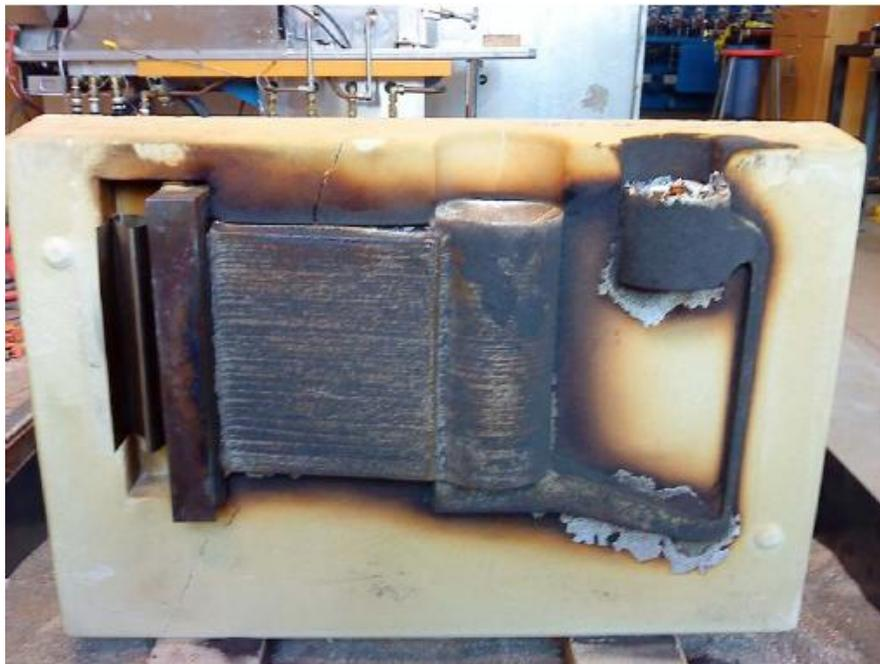
Figure 4.7: Solidified wedge, solid chill condition
