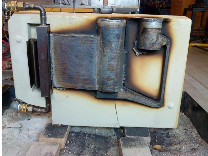
Figure 4.6: Solidified wedge, water cooled chill condition
