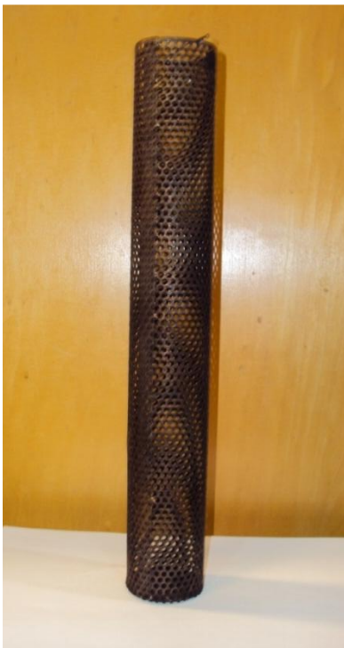
Figure 3 Steel basket used to conduct pretreatment experiments without explosive decompression
